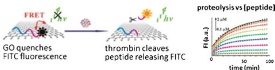
Figure 2.2.: Analytical devices based on biomolecule-graphene interfaces. (a) Functionalized graphene interface conductivity changes in response to bacterial binding. (b) A graphene oxide ( GO )-peptide sensor monitors protease activity on the basis of an increase in fluorescence as fluorescein isothiocyanate ( FITC ) is released after peptide cleavage by thrombin. ( CFU ) colony-forming units, ( FI ) fluorescence, ( FRET ) fluorescence resonance energy transfer, ( IV ) intravenous. (Adapted with permission from [134,137].)
