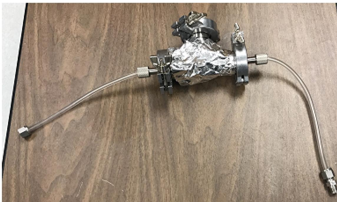
Figure 3.13. Collection Chamber used in the experiment, wrapped with aluminum foil
