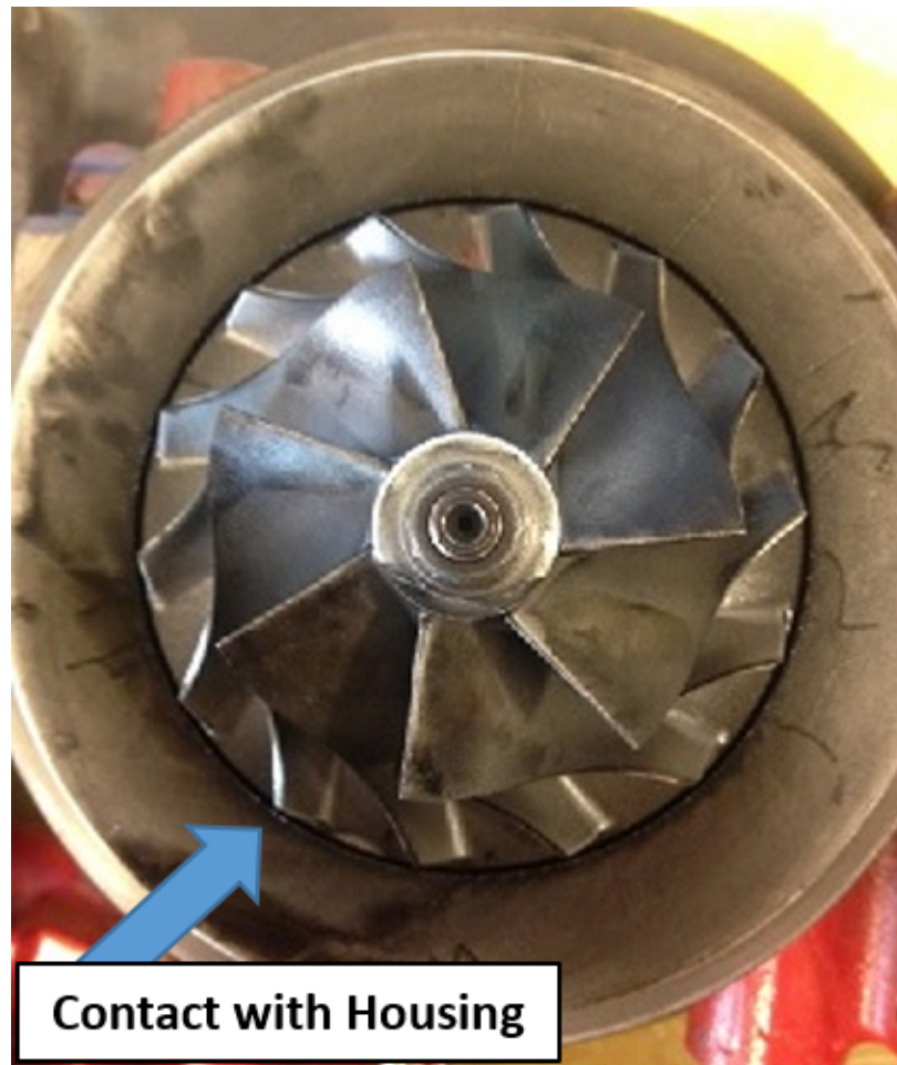
Figure 4.3. Intermittent compressor wheel contact with the compressor housing was caught before catastrophic failure of the blades.
