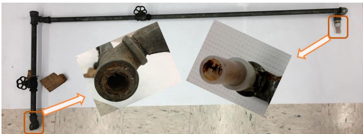
Figure B.2 Image of metal scales on exhumed galvanized and PEX-A drinking water pipes from the cold city water supply line.
