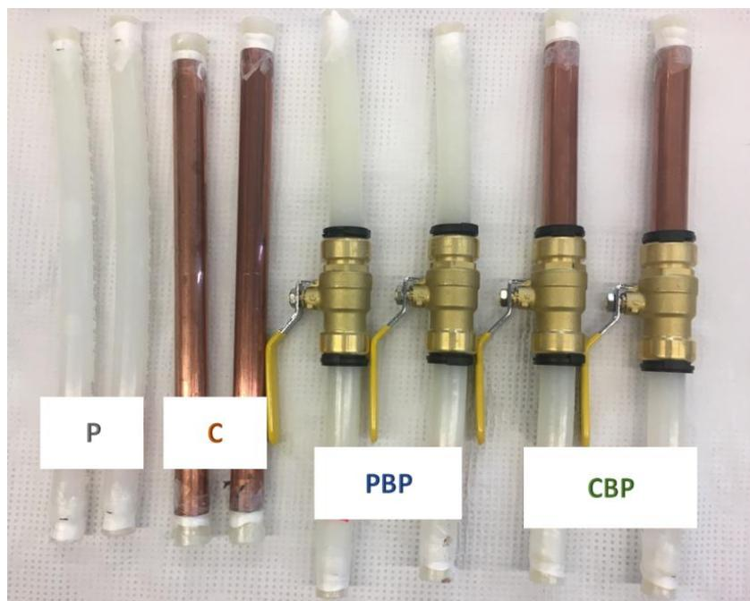
Figure B.1 Illustration of pipe apparatus and experimental groups' layout: (1) P rig: PEX pipe only (1.905 cm diameter, 30 cm length), (2) C rig: copper pipe only (1.905 cm diameter, 30 cm length), (3) PBP rig: PEX pipe (1.905 cm diameter, 15 cm length) + brass valve + PEX pipe (1.905 cm diameter, 15 cm length) and (4) CBP rig: copper pipe (1.905 cm diameter, 15 cm length) + brass valve + PEX pipe (1.905 cm diameter, 15 cm length). Only 2 of the 4 replicates are shown.
