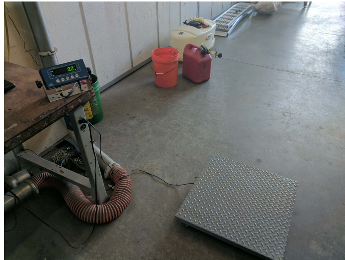
Figure 2.3. Weighing scale used to calibrate the weight of the fuel tank.
