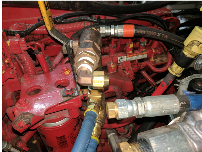
Figure 2.12. Return valve - Only one fuel pipe connected.
