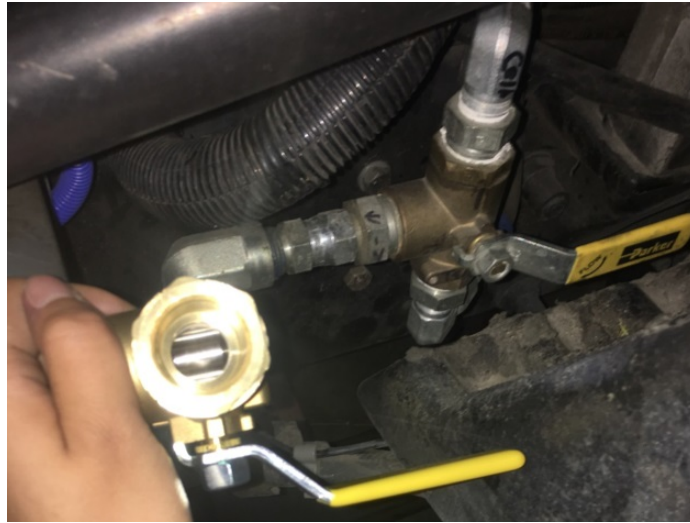
Figure 2.10. Three-way valve used to shift plumbing connection to the engine.
