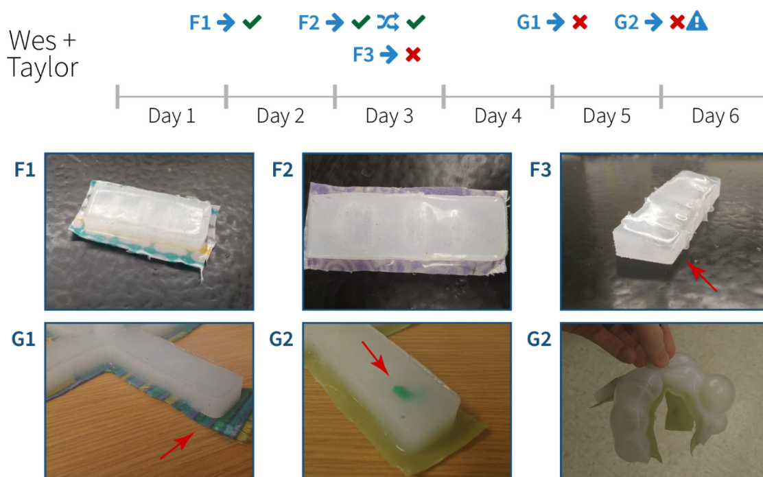
Figure 17. Snapshot of design successes and failures for Wes and Taylor. Finger and gripper attempts are abbreviated F and G, respectively. Iterations of each artifact type are numbered sequentially. Time for fabrication is indicated by the span of the arrow. Outcomes are marked as success (✓), partial success (⚠), or failure (✕). Reconfigured testing is indicated (✕). Repair attempts are indicated in turn.
