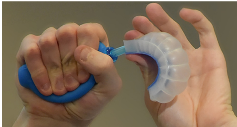
Figure 2. Soft robot finger inflation demonstration showing curved motion. Due to layer flexibility differences and internal air pressure, the gripper actuation is constrained to a curve.
