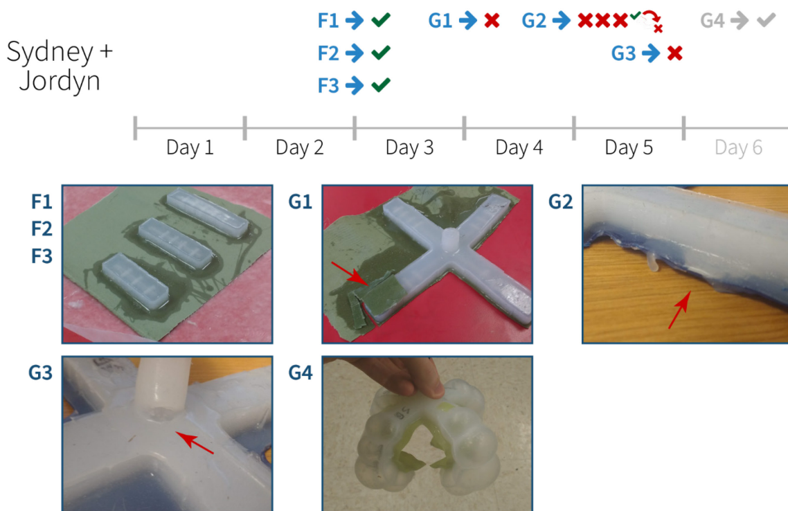
Figure 14. Snapshot of design successes and failures for Sydney and Jordyn. Finger and gripper attempts are abbreviated F and G, respectively. Iterations of each artifact type are numbered sequentially. Time for fabrication is indicated by the span of the arrow. Outcomes are marked as success (✓) or failure (✗). Instances of momentary success are marked by a transition from success to failure. Repair attempts are indicated in turn. In order to build a successful solution, the team persisted after I stopped observing; this day is included in the timeline.
