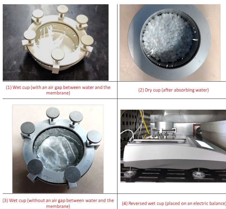
Figure B.3 (1) Wet cup, (b) dry cup, (c) fulfilled wet cup, and (d) liquid desiccant cup (photos credit to Xiaobing Liu, ORNL).
