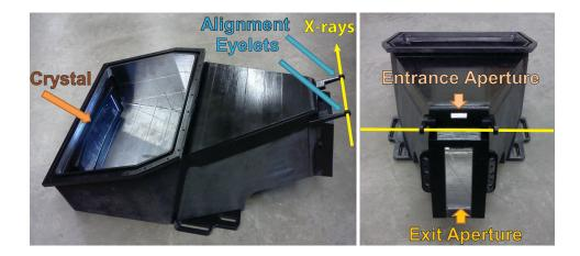
Figure 4.6. A new 3-D printed spectrometer is shown with the crystal mounted to the back face in the horizontal orientation, as shown, with two removable eyelets to align the spectrometer to the x-ray beam (left). A removable plate seals to the back half of the spectrometer to maintain a He environment and allow access inside (plate not shown). The entrance and exit apertures are shown from the front without the internal shielding in place.
