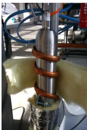
Figure 5.10: Copper tubing and insulation used to facilitate condensation of leftover vapor.
