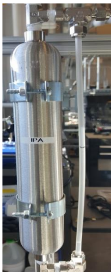
Figure 5.6: Supply cylinder for isopropanol with liquid level line installed.
