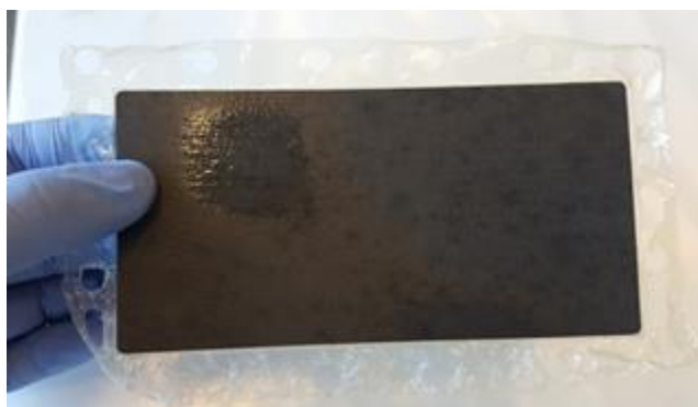
Figure 6.10: SPEEK membrane after operation in alcohol electrochemical cell.
