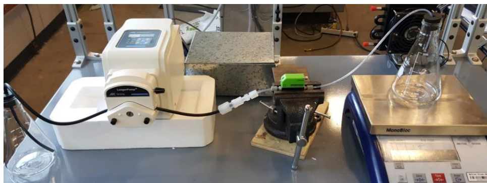
Figure 5.21: Calibration setup for liquid flow meters.
