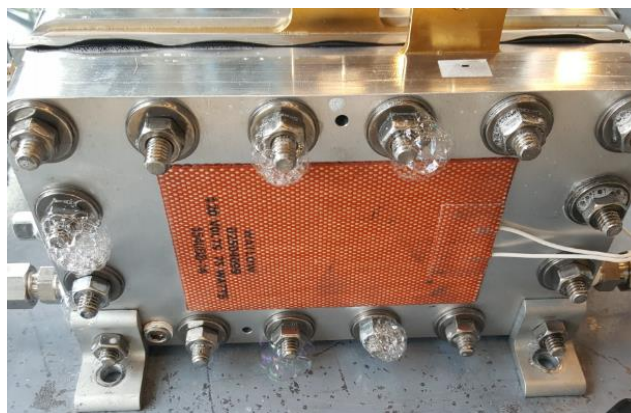
Figure 7.4: Cell leakage using 20 cm 2 flow fields.
