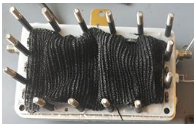
Figure 6.3: Swollen membrane after operating cell using alcohol.
