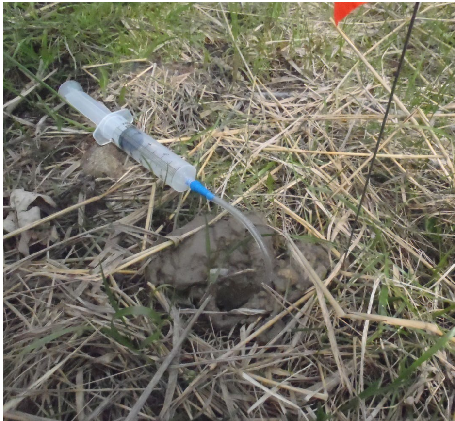
Figure 3. Hand pump constructed from tubing, a catheter adapter, and a syringe inserted into crayfish burrow to draw water from crayfish burrows.
