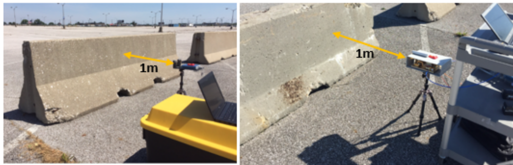
Fig. 4.61. Concrete divider measurement using 24GHz (left) and 77GHz (right) Radar
