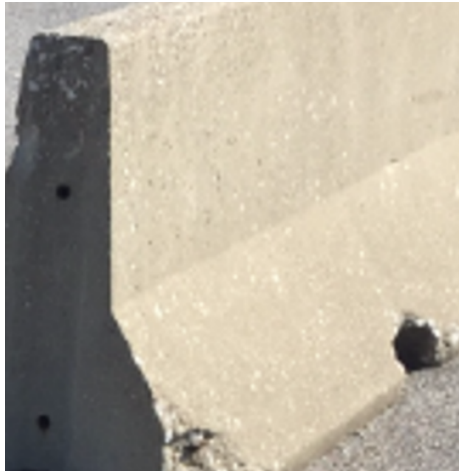
Fig. 4.72. Gravels visible on the surface of concrete divider sample 2
