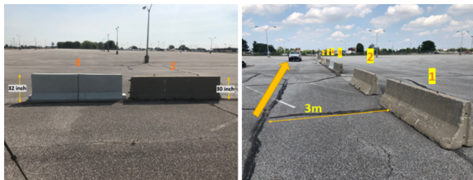
Fig. 5.26. Concrete divider surrogate is placed between real concrete dividers
