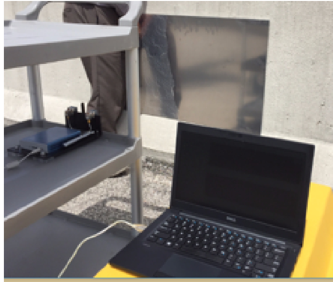
Fig. 4.60. Reflectivity calibration using an aluminum plate
