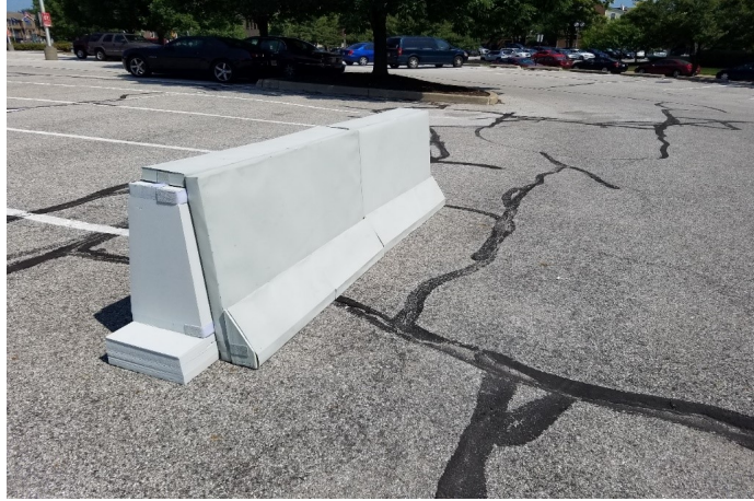
Fig. 5.23. Final surrogate concrete divider
