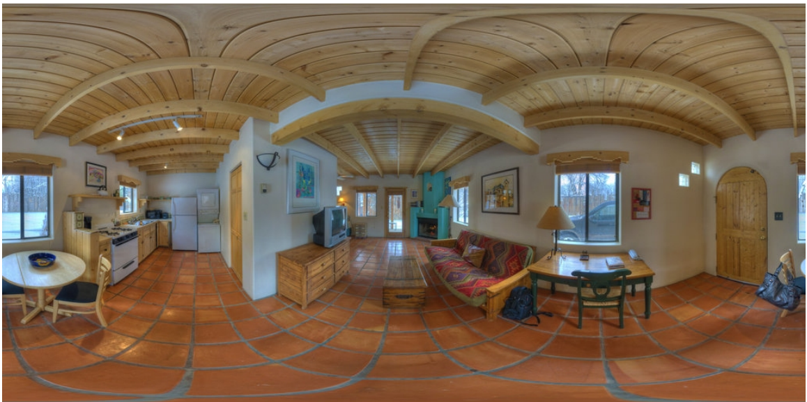
Fig. 3.4. Example of an environment map captured with a 360 degree panoramic camera, a similar image could be generated using a mirrored ball.
