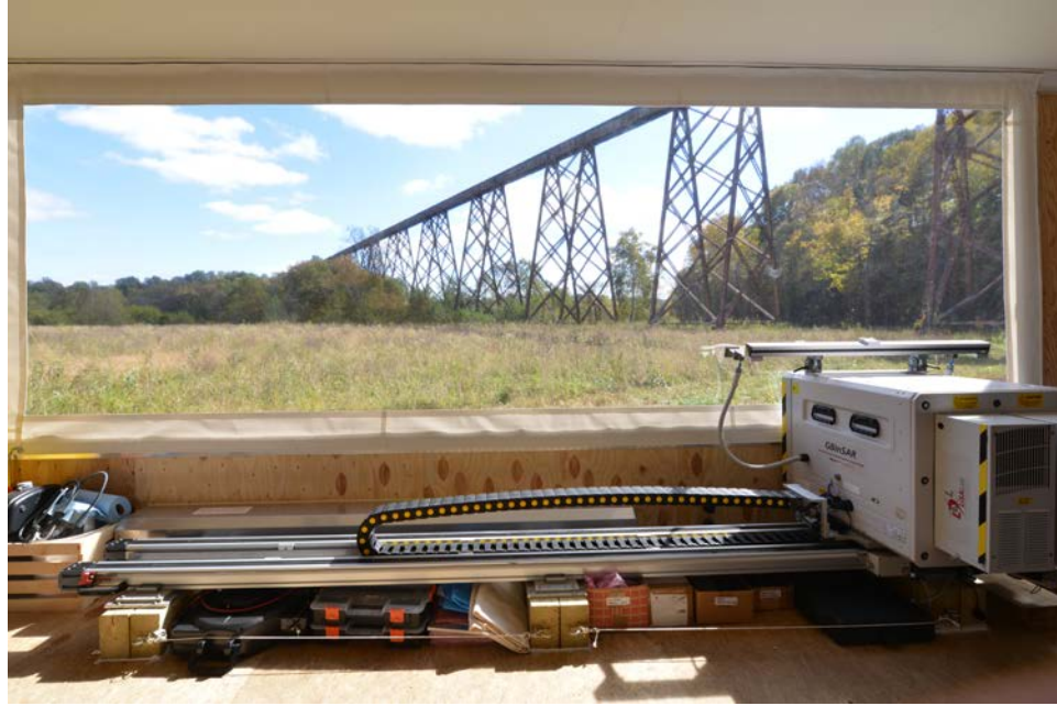
Figure 2.3. A photo showing GBSAR system by LiSALAB
