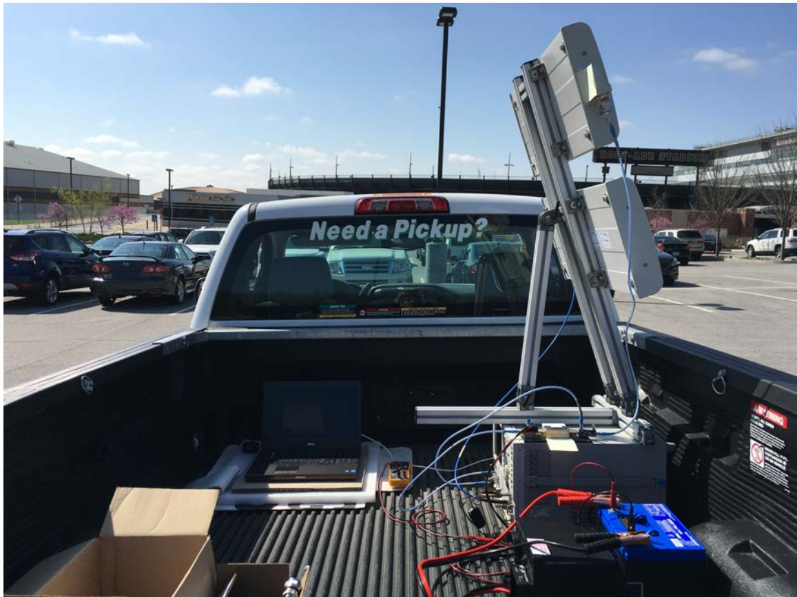
Figure 4.3. Modified VNA-based SAR system installed on truck
