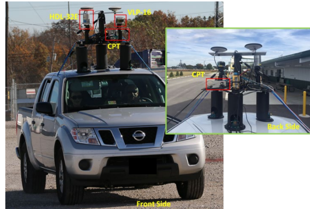
Figure 5.1. Terrestrial mobile mapping system used in this thesis
