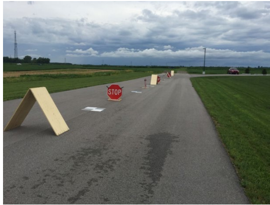
Figure 5.4. Calibration test field with hut-shaped targets and highly reflective boards
