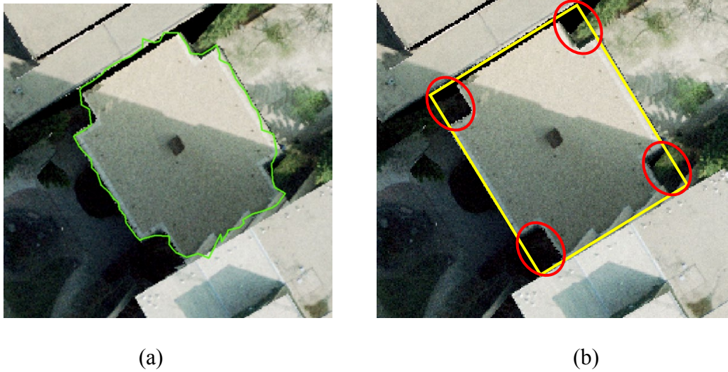
Figure 4.5. Illustration of incorrect building model as a result of inappropriate Th_{pt} value: (a) extracted boundary and (b) shape of building model
