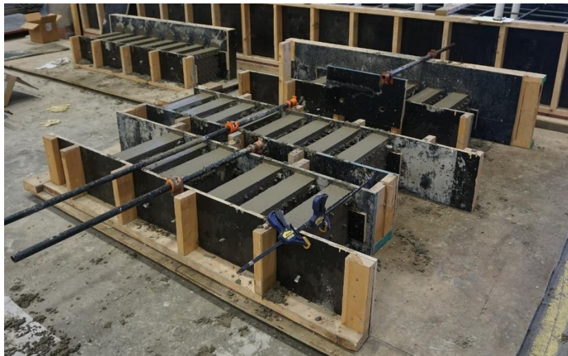
(b) Specimens after concrete casting
