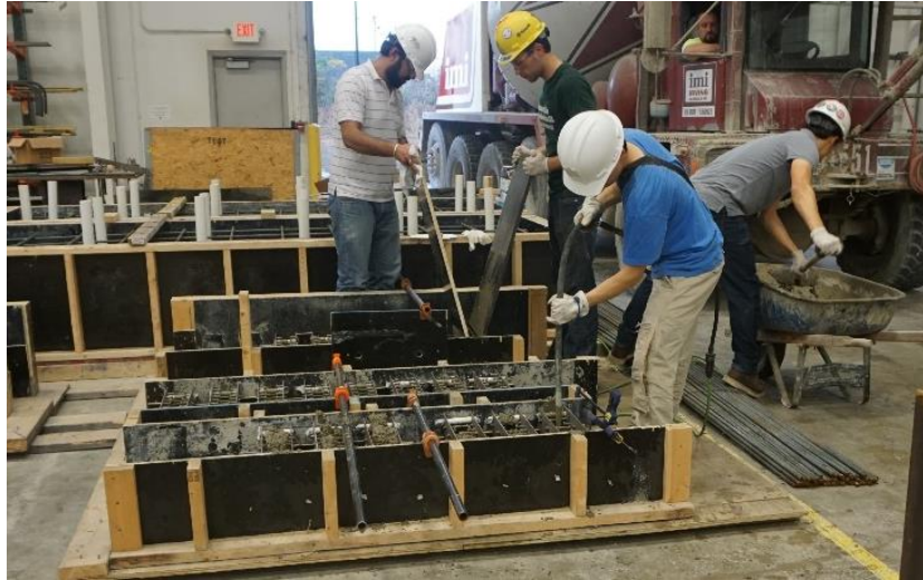
(a) Specimens during concrete casting
