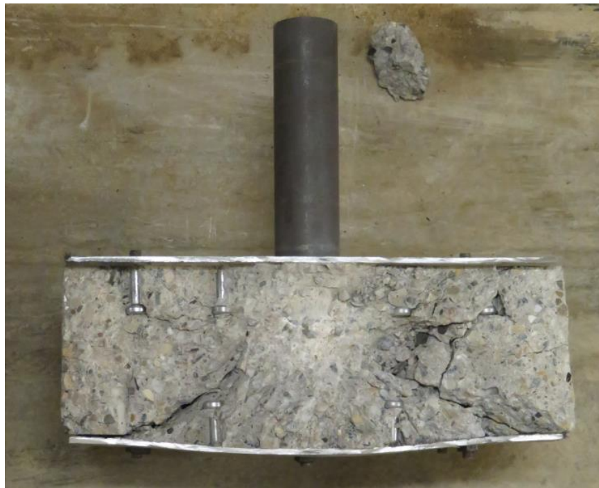
Figure 4-29 Photograph of damage in a cross-section cut from the post-test specimen: Gr.2 #3
