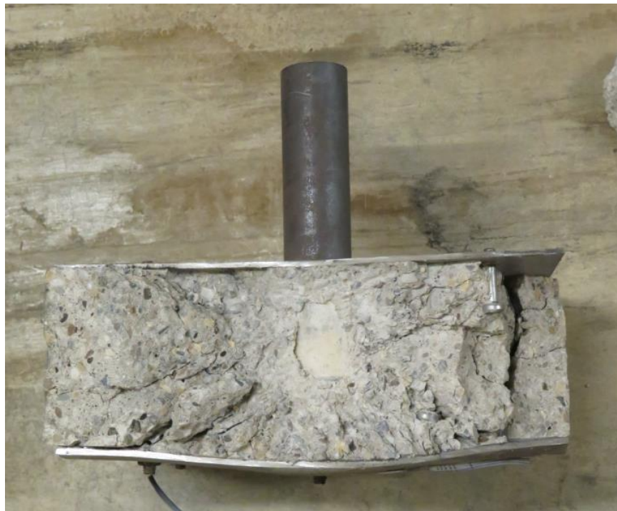
Figure 4-30 Photograph of damage in a cross-section cut from the post-test specimen: Gr.2 #4
