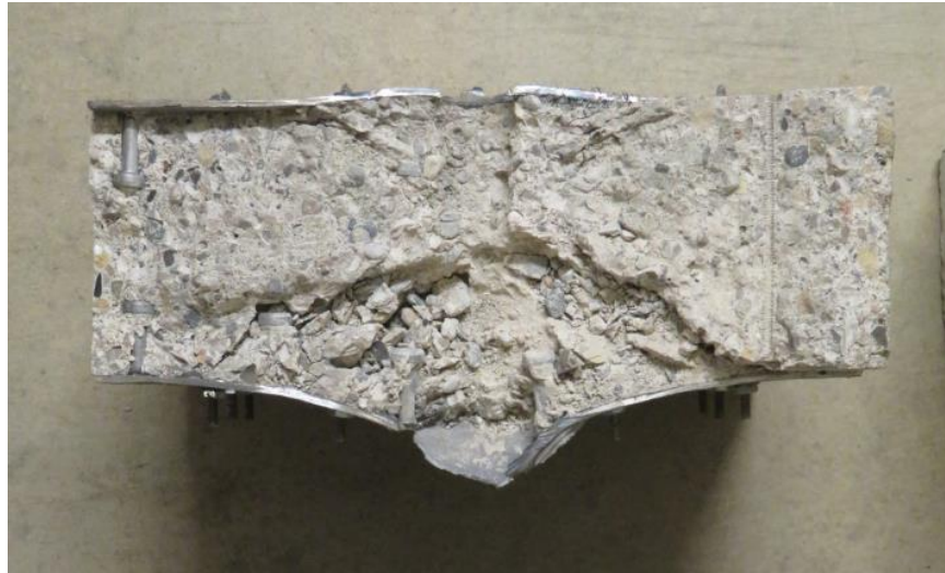
Figure 4-24 Photograph of damage in a cross-section cut from the post-test specimen: Gr.1 #8
