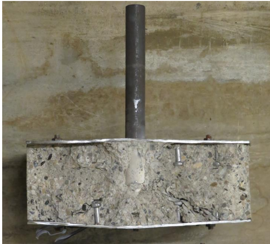
Figure 4-27 Photograph of damage in a cross-section cut from the post-test specimen: Gr.2 #1
