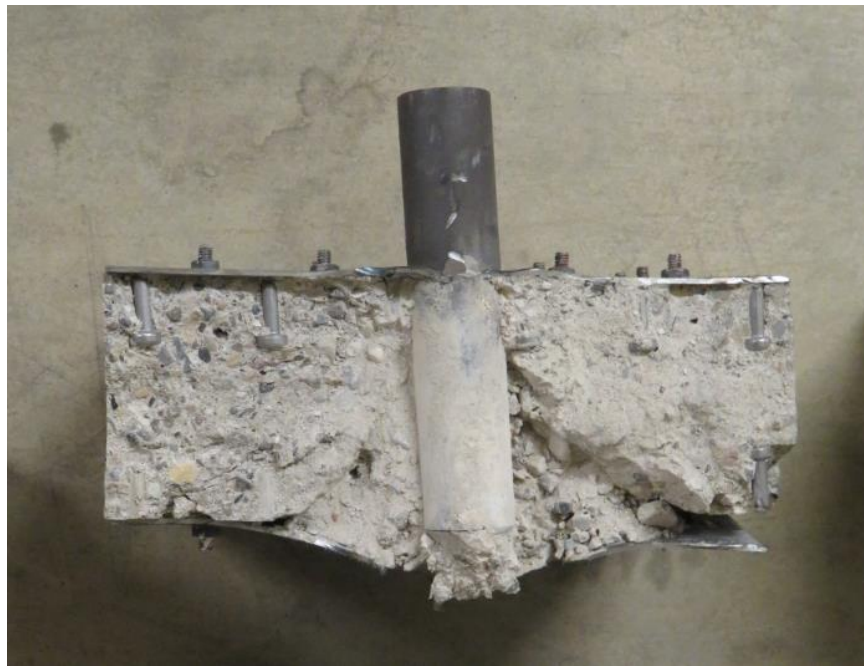
Figure 4-25 Photograph of damage in a cross-section cut from the post-test specimen: Gr.1 #9
