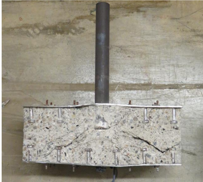
Figure 4-19 Photograph of damage in a cross-section cut from the post-test specimen: Gr.1 #3
