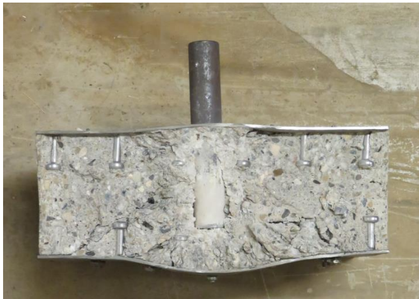
Figure 4-18 Photograph of damage in a cross-section cut from the post-test specimen: Gr.1 #2
