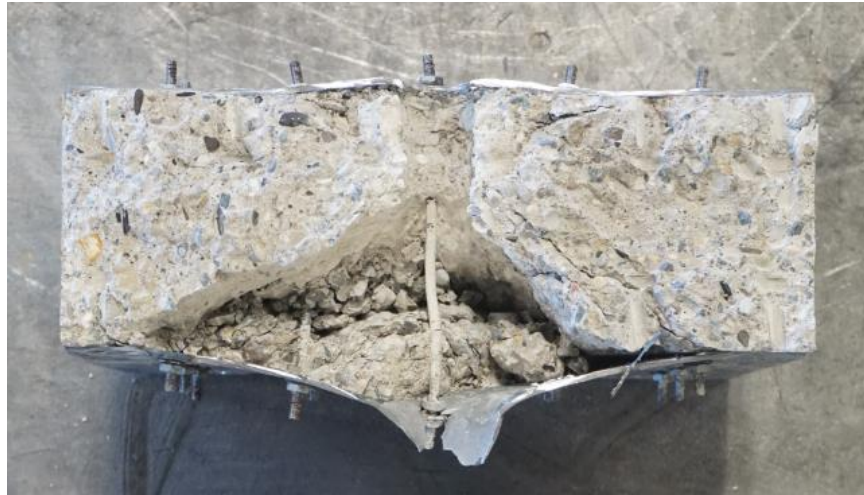
Figure 4-23 Photograph of damage in a cross-section cut from the post-test specimen: Gr.1 #7
