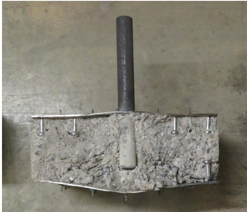
Figure 4-31 Photograph of damage in a cross-section cut from the post-test specimen: Gr.3 #1
