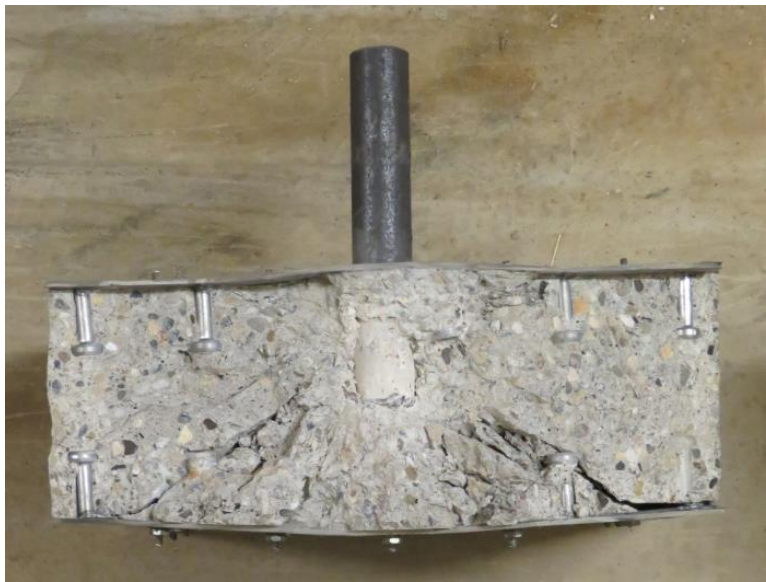
Figure 4-17 Photograph of damage in a cross-section cut from the post-test specimen: Gr.1 #1
