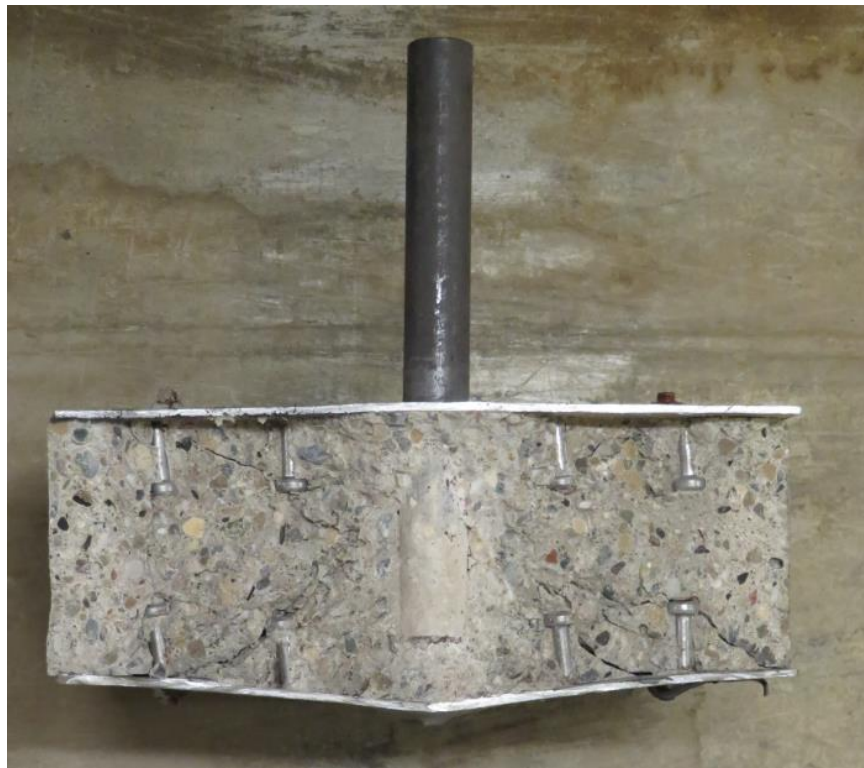
Figure 4-28 Photograph of damage in a cross-section cut from the post-test specimen: Gr.2 #2
