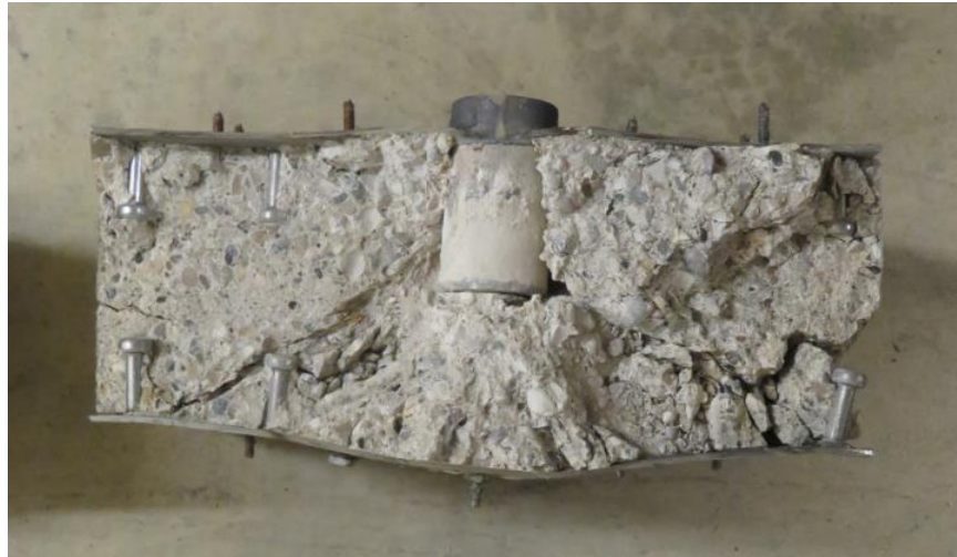
Figure 4-22 Photograph of damage in a cross-section cut from the post-test specimen: Gr.1 #6
