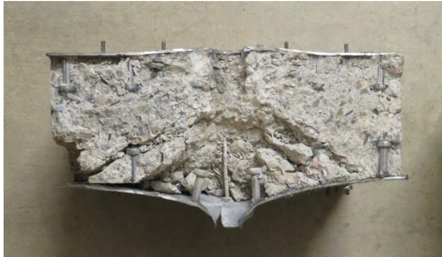
Figure 4-32 Photograph of damage in a cross-section cut from the post-test specimen: Gr.3 #2
