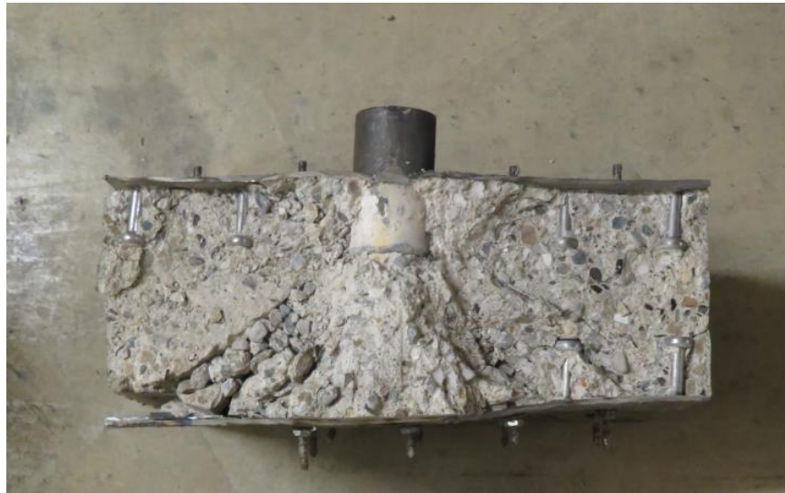
Figure 4-21 Photograph of damage in a cross-section cut from the post-test specimen: Gr.1 #5
