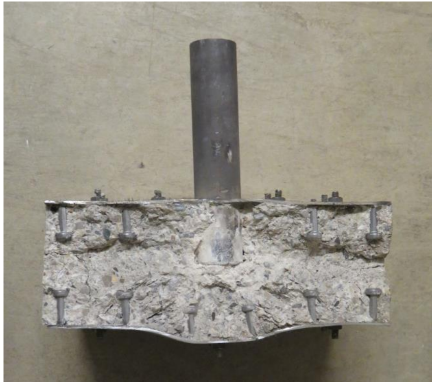
Figure 4-26 Photograph of damage in a cross-section cut from the post-test specimen: Gr.1 #10
