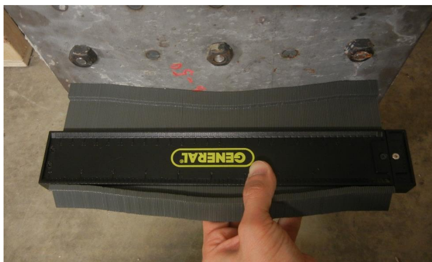
Figure 3-14 Bulging depth measurement using a contour gage after test
