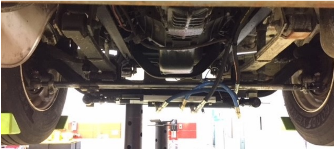
Figure 7.18. Cylinder Installation on Vehicle
