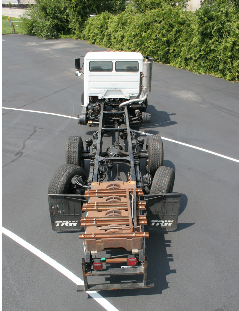
Figure 7.28. Rear Axle Steering System on Test Vehicle
