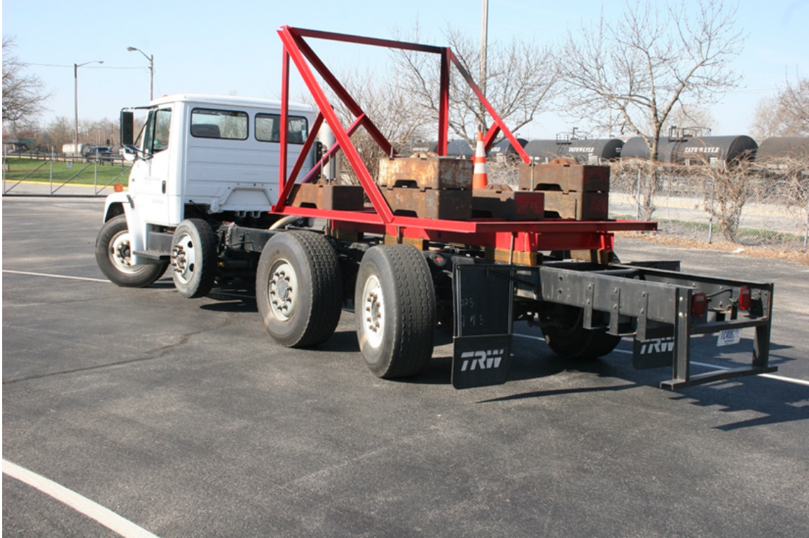
Figure 6.7. Test Vehicle Equipped with Rear Axle Steering System
