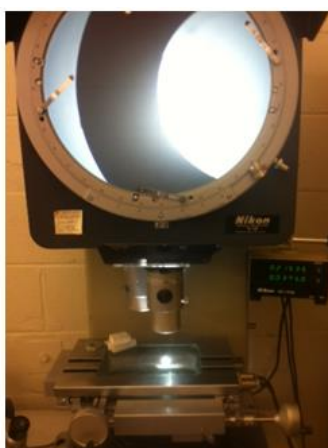
Figure 5.2 Nikon Profile Projector V-12 used to measure the diameters of the o-ring seals.
