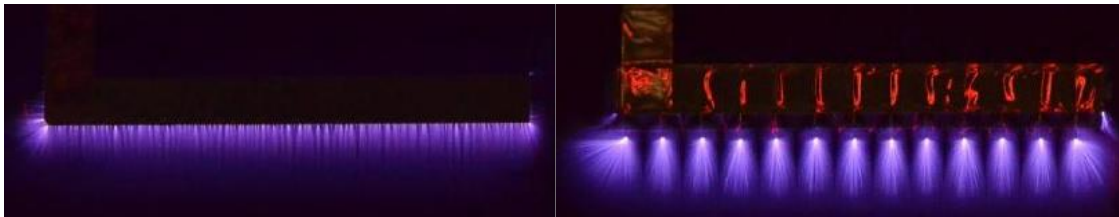
Figure 3.6: Plasma formation on conventional DBD actuator layout (left) and on comb-shaped DBD actuator layout (right) at a repetition frequency of 100 Hz [63].
