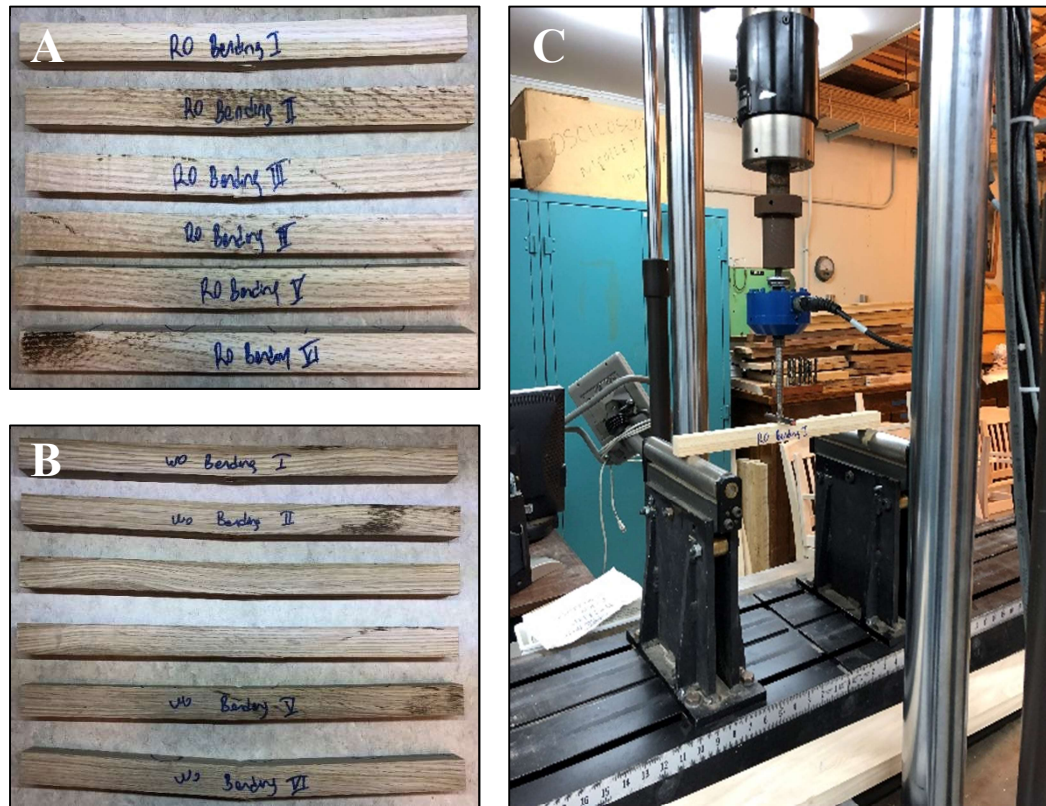
Figure B.2 A. Red Oak Samples, B. White Oak Samples and C. Test Set-Up
