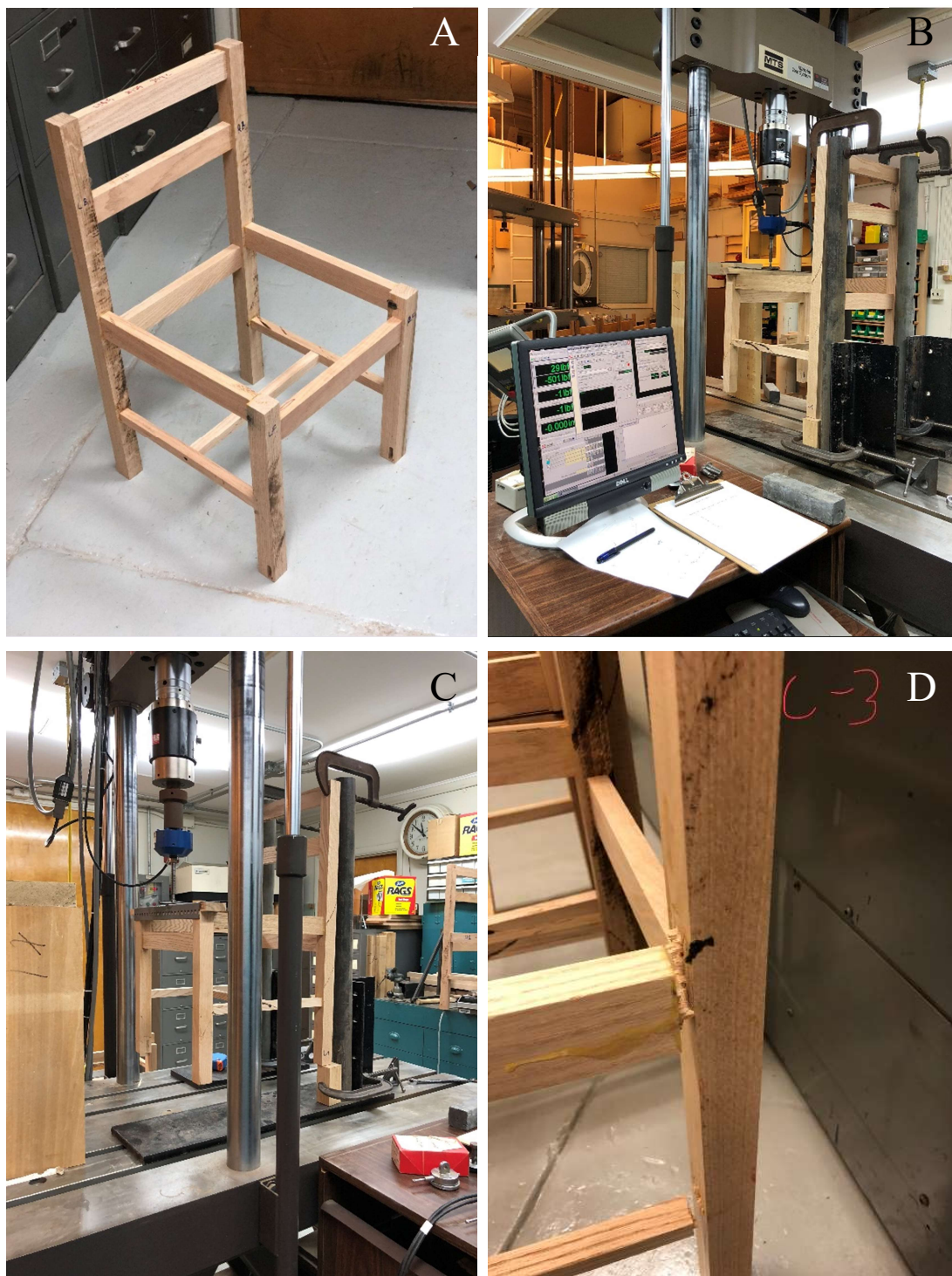
Figure B.3 Chair Sample for Static Load Test and Typical Joint Failure
