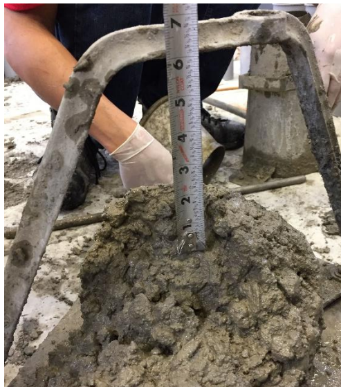
(a) Slump Test
