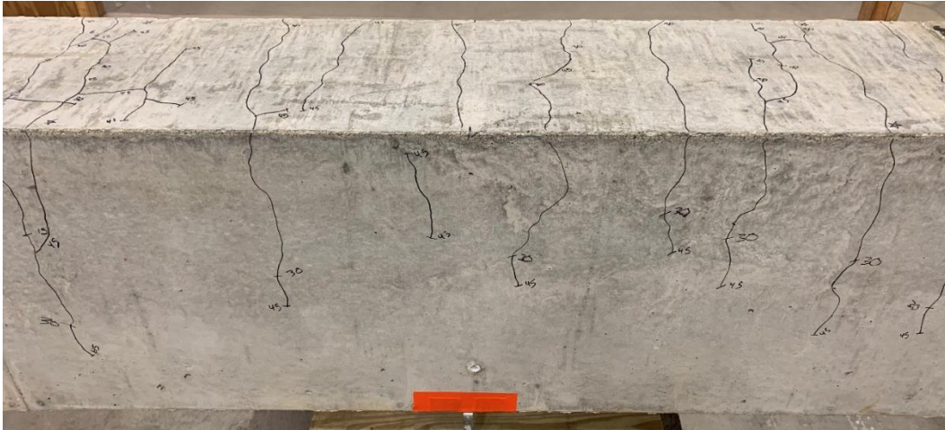
Figure 5.4: Typical Flexural Cracking within Confined Splice Region (C3/60-40-5-200)
