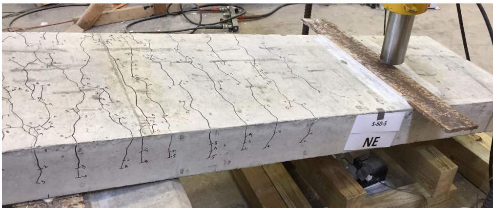
Figure 3.10: Post-Failure Shear Span Cracking (S-60-5)
