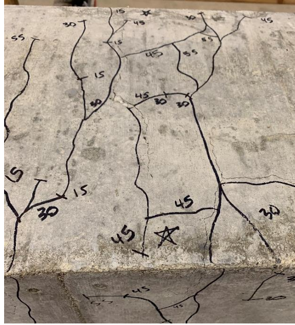
Figure 5.23: Longitudinal Crack Branching (C3/60-50-5-200)
