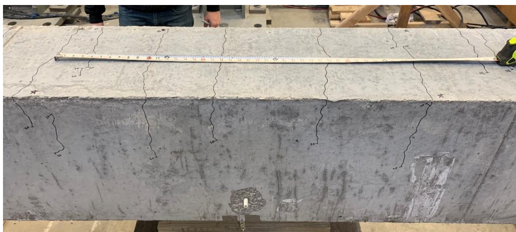
Figure 5.9: Transverse Flexural Cracking within Splice Region (C3/60/2-40-10-50)
