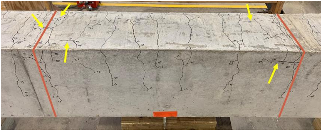
Figure 5.15: Longitudinal and Branch Cracking Before Flexural Failure (C3/60-50-5-200)
