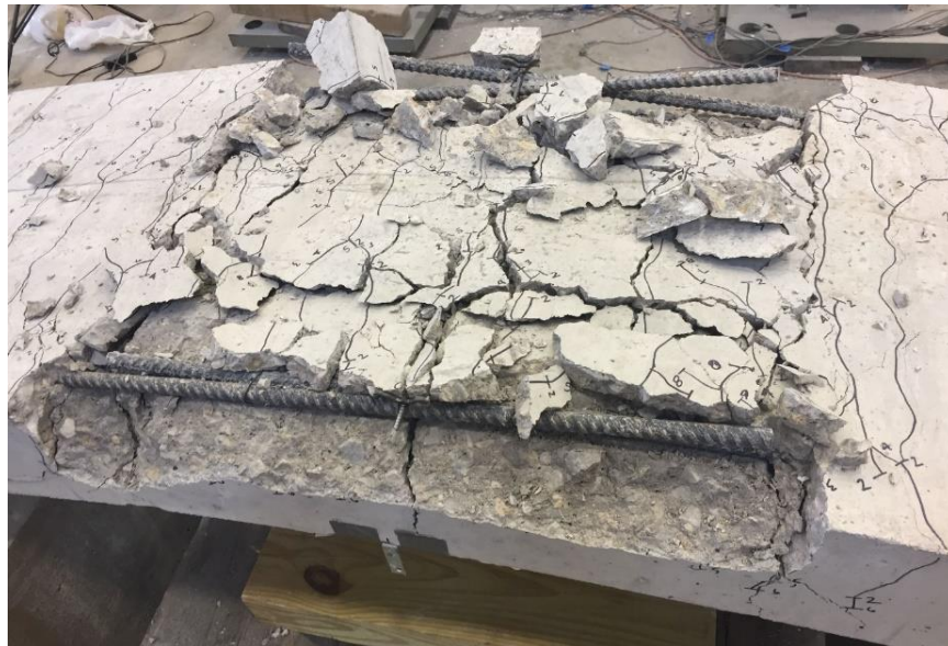
Figure 3.13: S-40-5 Face- and Side-Splitting Failure
