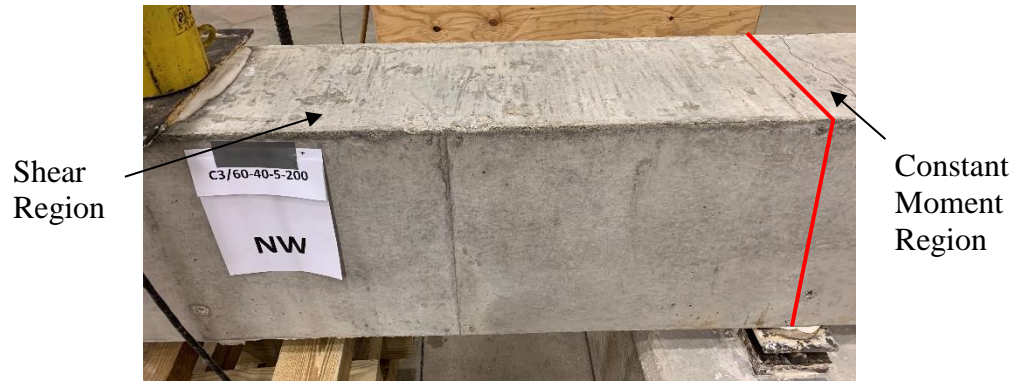
Figure 5.11: Shear Span – Early Testing (C3/60-40-5-200)
