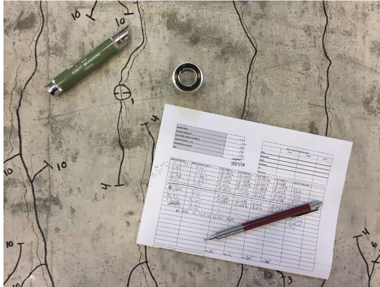
Figure 2.30: Crack Width Microscope and Mapping Process
