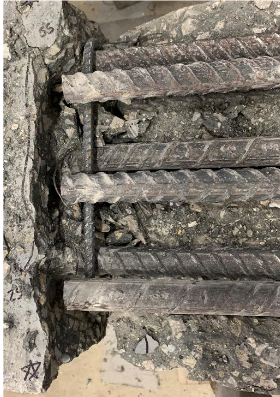
Figure 5.20: Bar Slip on Specimen C3/60/2-40-10-25
