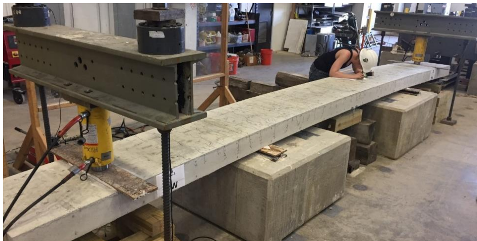
Figure 2.32: General Slab Test – Crack Mapping (S-80-5)
