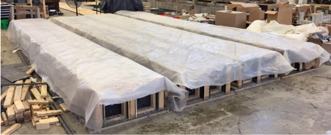
Figure 4.29: Series VI Moist Curing – Plastic Cover
