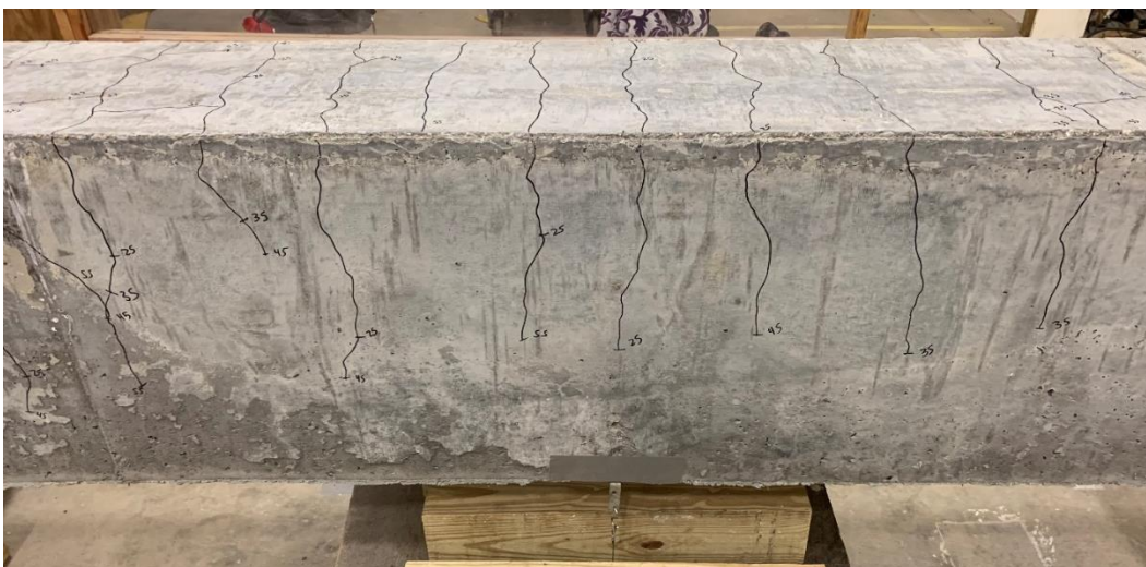
Figure 5.3: Typical Flexural Cracking within Unconfined Splice Region (U-60-10)
