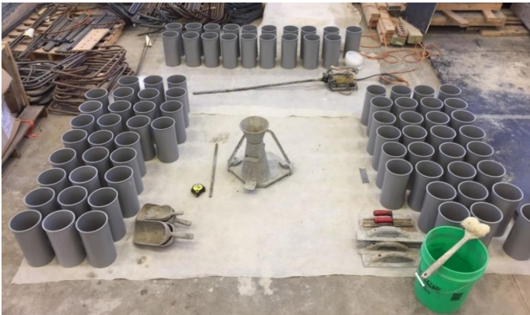
Figure 2.14: Typical Concrete Cylinder Preparation Space
