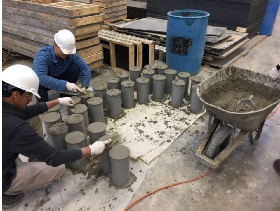
Figure 2.15: Series V Cylinder Casting
