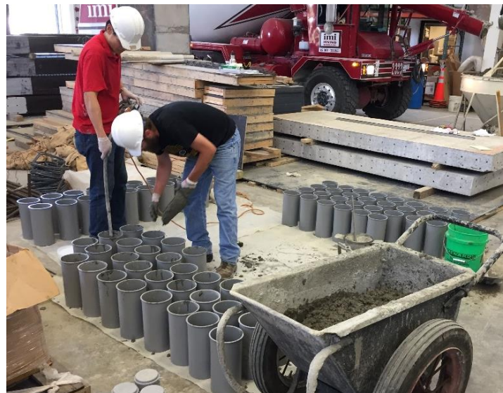
(b) Cylinder Casting Space
