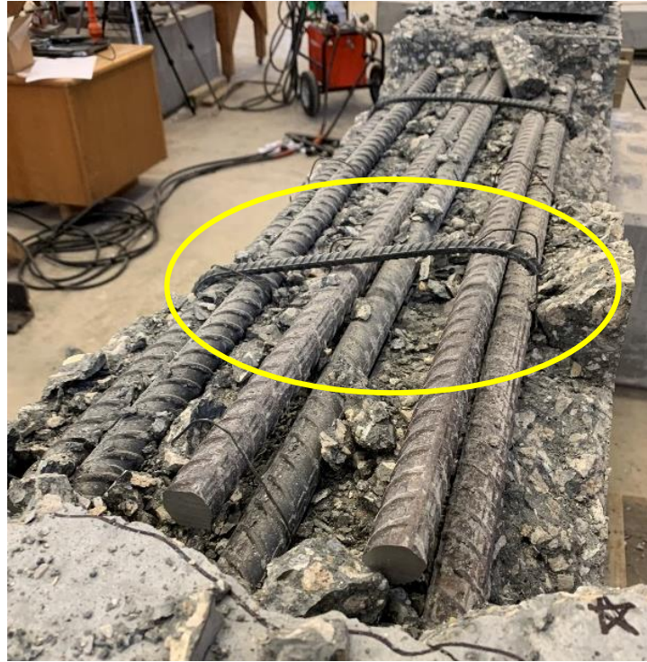
Figure 5.22: Ruptured Stirrup on Specimen C3/60/2-40-10-50
