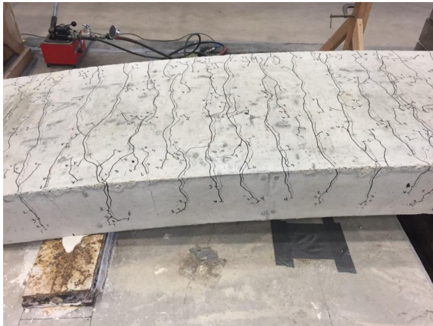
Figure 3.4: Typical Flexural Cracking – West Side and Tension Face (S-80-5)
