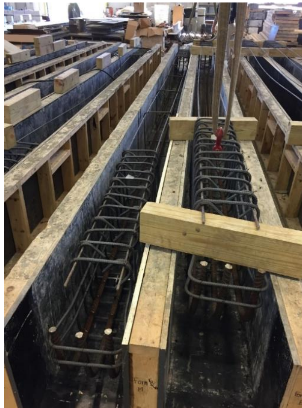
Figure 4.18: Beam Shear Region and Cage Lifting
