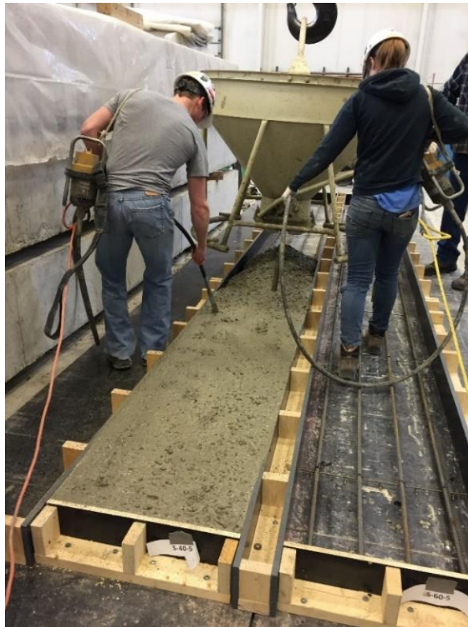
Figure 2.16: Series V Consolidation Process
