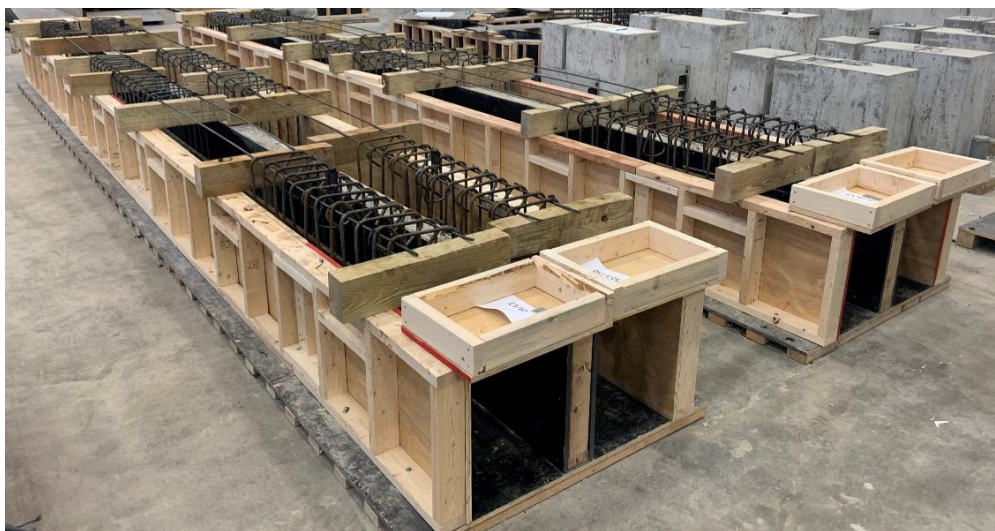
Figure 4.16: Series VII Cage Support Blocks
