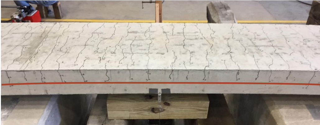
Figure 3.9: Side Crack Propagation (S-100-5)
