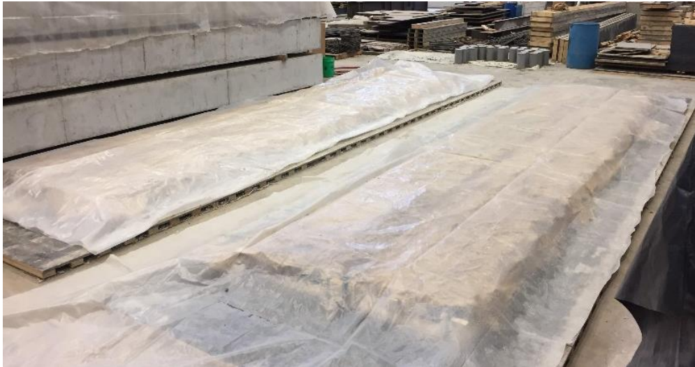
Figure 2.19: Series V Moist Curing
