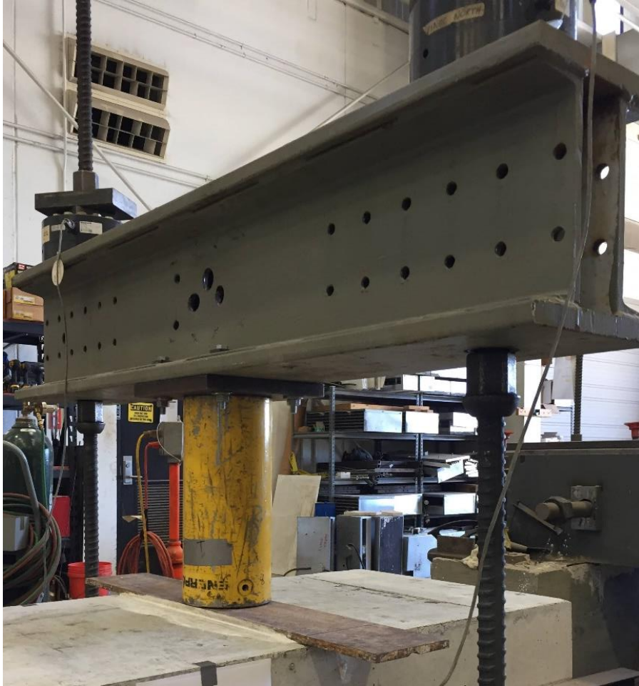
Figure 2.24: Typical Crossbeam Setup
