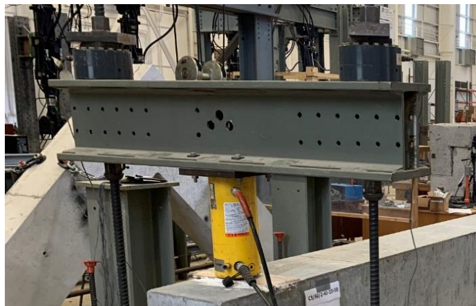
Figure 4.33: Typical Crossbeam Setup
