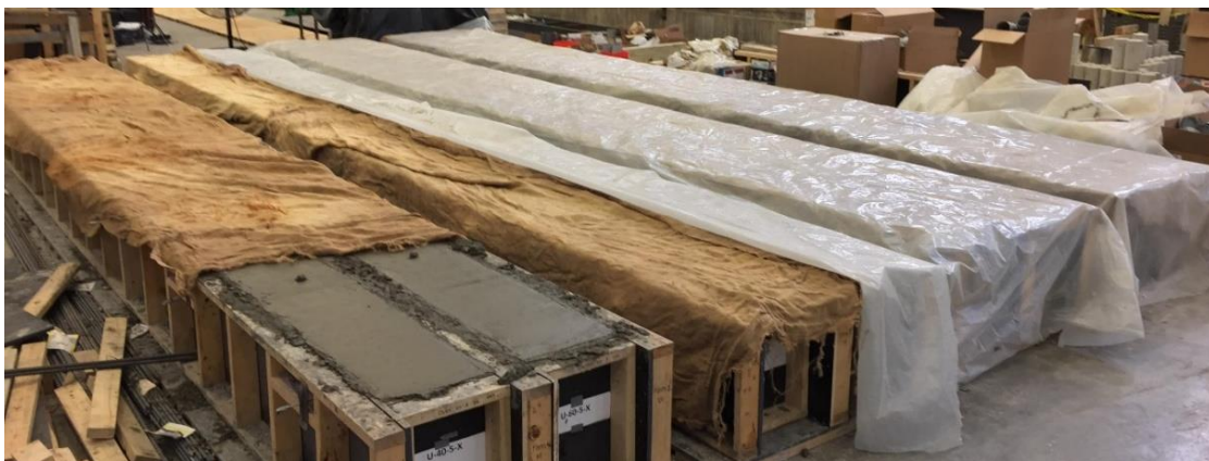
Figure 4.28: Series VI Moist Curing – Burlap Cover
