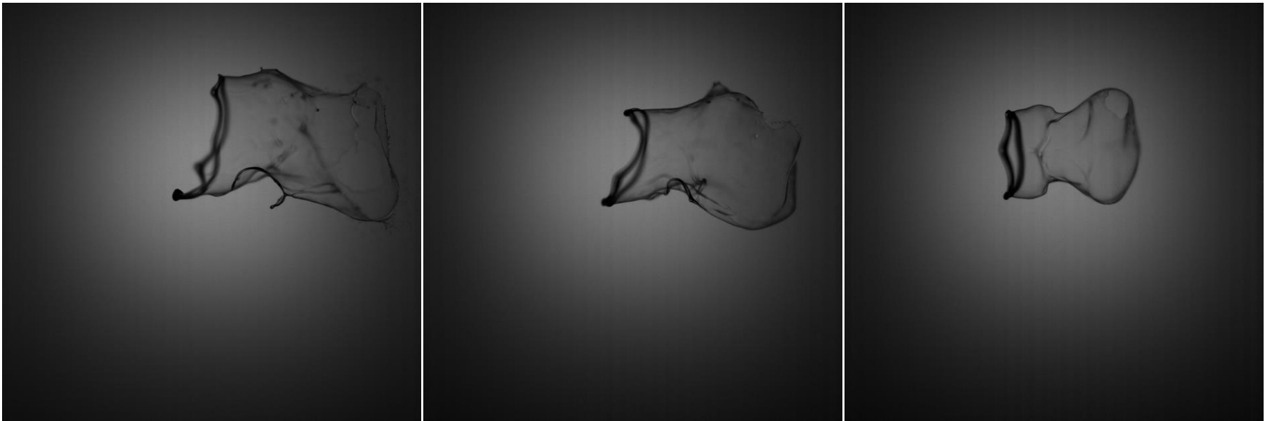
Figure 5.2 Shadowgraph of ethanol drop at We=20 , U=0, 1 and 2 kV from left to right
