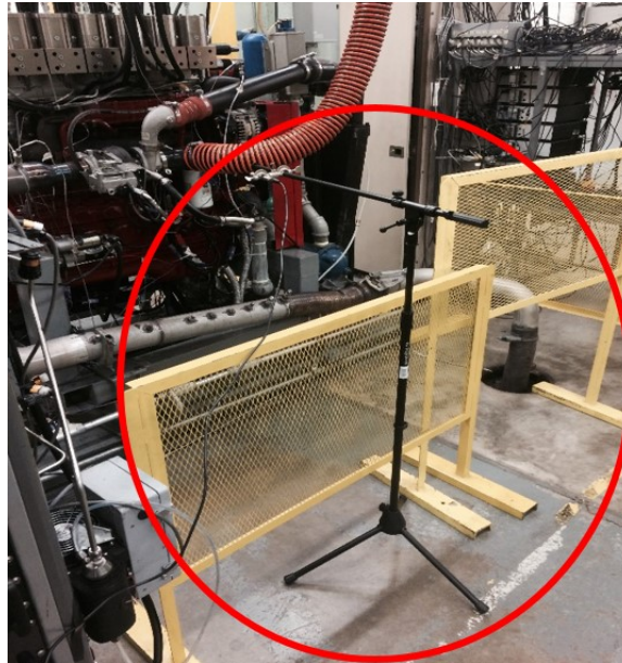
Figure 5.27. Microphone setup for acoustic testing of the engine.
