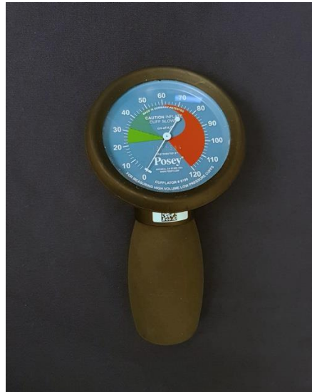
Figure 3.3: A Posey Cufflator™ is an ETT cuff-specific aneroid manometer which can measure the ETT cuff pressure between 0 to 120 cmH 2 O. The ETT cuff pressure can be adjusted by compressing the inflator bulb for increasing pressure and the red air vent button at the back for releasing the excessive air. Note the color areas on the faceplate. The green area represents acceptable cuff pressure range whereas the red area indicates high ETT cuff pressure.
