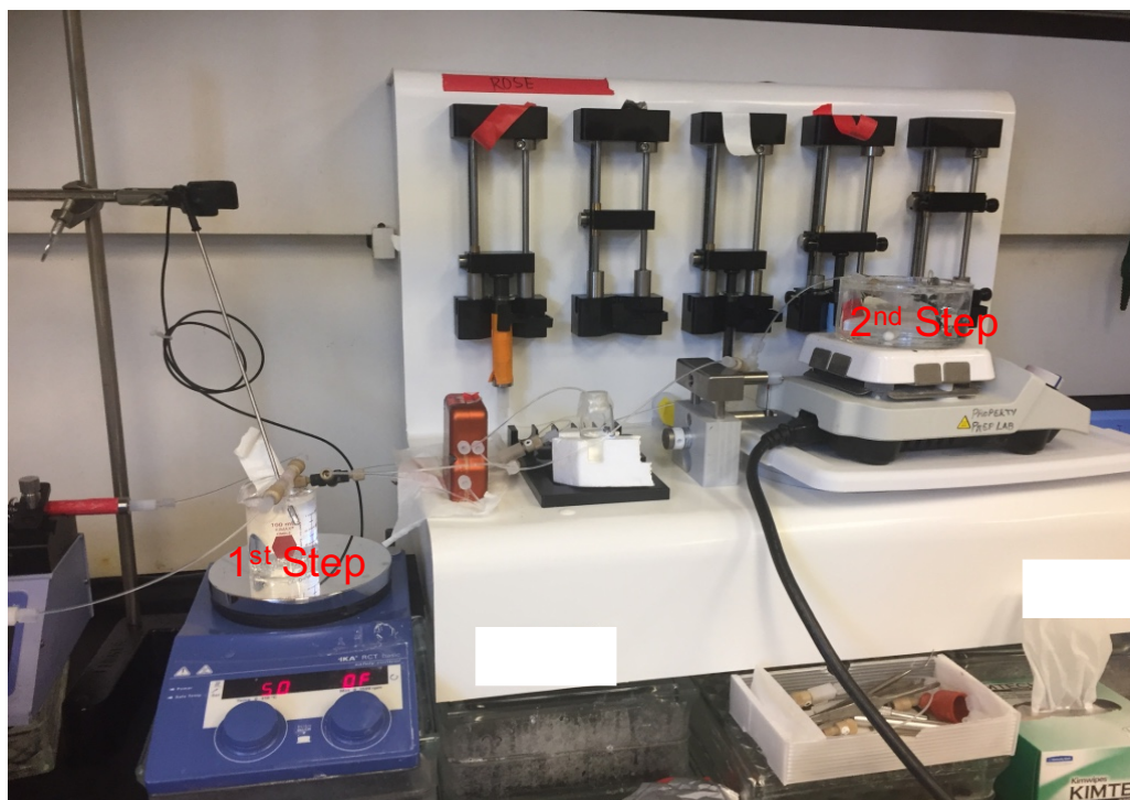
Figure C14: Telescoped lomustine synthesis using TBN as a nitrosation reagent, before reaction initiation.
