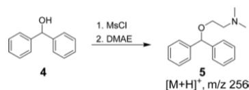
Scheme 2. Mesylation of 4 followed by reaction with 2-(dimethylamino)ethanol (DMAE) to form diphenhydramine ( 5 ).
