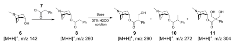
Scheme 3. Esterification reaction of 6 with 7 to synthesize 8 followed by base-catalyzed aldol condensation with formaldehyde to synthesize atropine ( 9 ).
