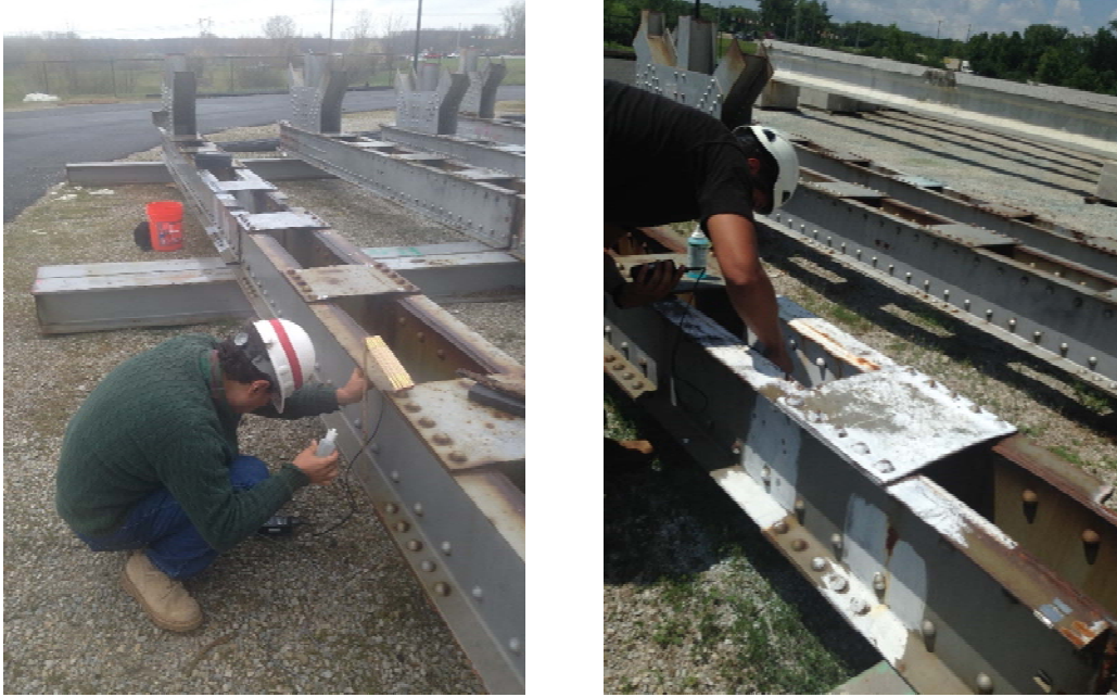
Figure 6.4 Inspectors taking thickness measurements of the truss chord
