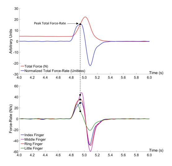
Fig. 2.2: Data from a representative IMRL trial. Participant produced a rapid increase in force and then relaxed to a rested state (up-pulse trial). At the instant of total peak force-rate, the force-rate for each finger was identified.
