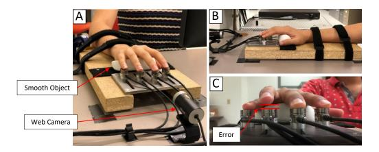
Fig. 2.1: Front view (A), side view (B), and web camera view (C) of the experimental setup. The web camera was used to observe errors and a smooth object was placed under the hand to maintain a consistent hand configuration.
