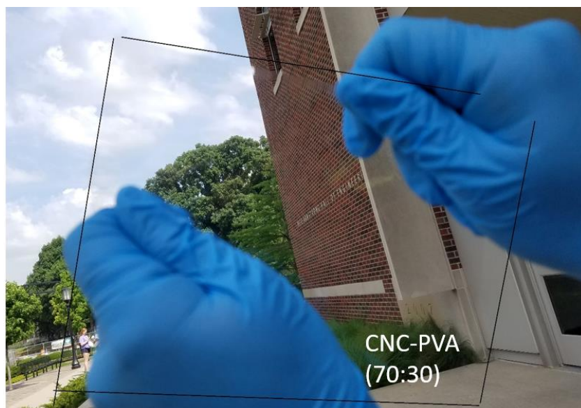
Figure BS7: Total transparency of coated PET film with very low haze and high clarity. (Black dotted line for showing film outline.)
