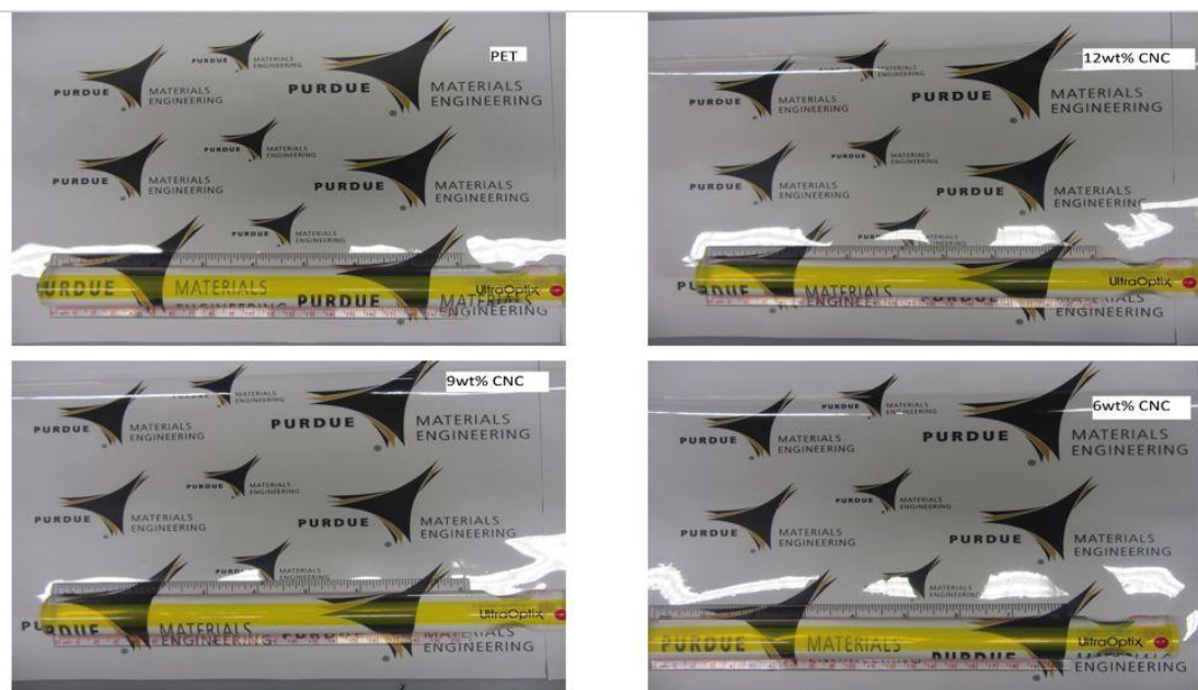
Figure 2.8 Photographs of CNC coatings on PET substrate (15cmX15cm): (top left) PET substrate, (top right) 12wt% CNC solution, (bottom left) 9wt%, (bottom right) 6wt%.
