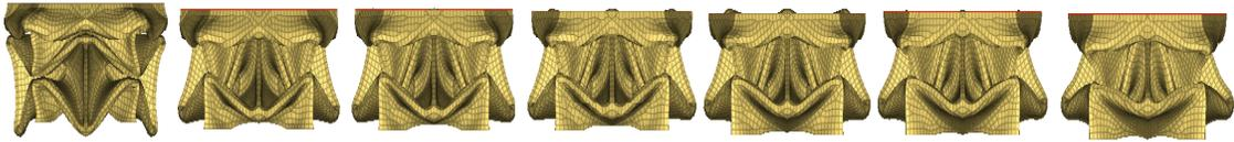
Fig. 4.14. All 7 Crushed Configurations of Origami with 2 Modules with  $\theta$  from  $140^\circ$  to  $170^\circ$
