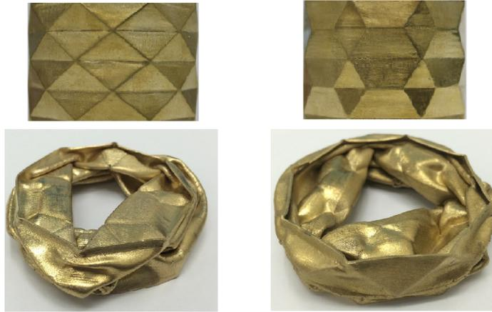
Fig. 2.21. Diamond (left) and Full Diamond (right) patterns by Yang [105]
