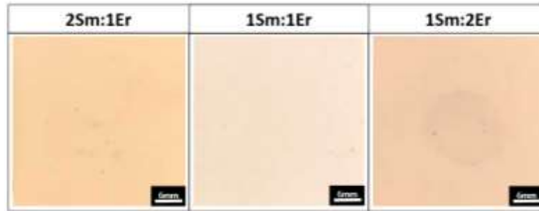
Figure 36. Optical images of the surface after the preparation in the oxygen furnace for the 2Sm:1Er, 1Sm:1Er, and 1Sm:2Er samples.
