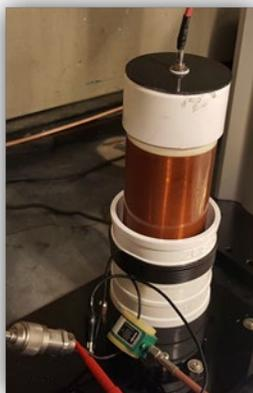
Figure 2.10: Custom air core resonance high voltage transformer.
