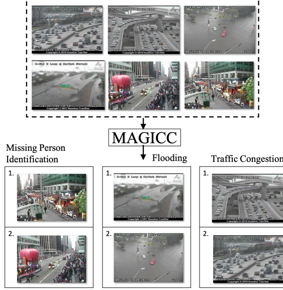
Figure 1.1. MAGICC: Method to Analyze Geotagged Images for Camera Classification takes input as a list of cameras, and a required computer vision application. It outputs a rank list of the most useful cameras for that particular application.
