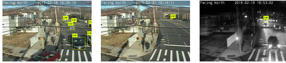
(a) Misses the red car in front (b) Wrongly predicts a car at night (c) Detects very few cars
