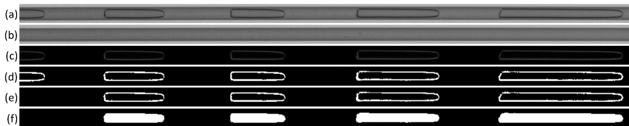
Figure 8.2. Selected frame showing the (a) original image, (b) background image, (c) gray-scale image after background subtraction, (d) binary image after thresholding, (e) binary image after removing partial bubble interfaces, and (f) final binary image with vapor bubbles filled in white.
