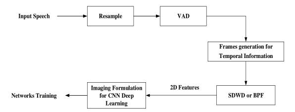
Figure 2.6 Two-dimension feature extraction and image generation.
