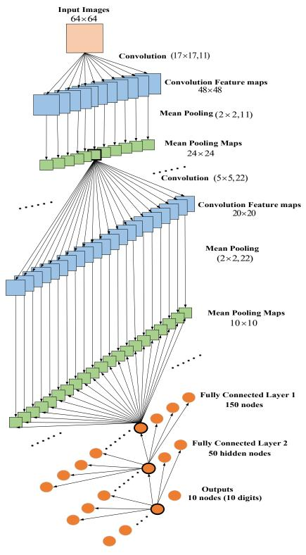
Figure 3.7 CNN structure.
