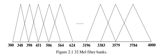
Note that there exist overlaps among filters as shown in Figure 2.1 due to the filter roll-off nature. For instance, the band 30 with the range from 3383.176 Hz to 3784.678 Hz has an overlapped frequency part with the band 31 from 3579.220 Hz to 4000.000 Hz.
