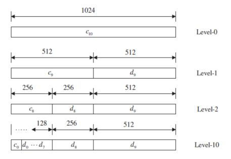
Figure 2.3 DWT coefficient layout for the ten-level decomposition.
