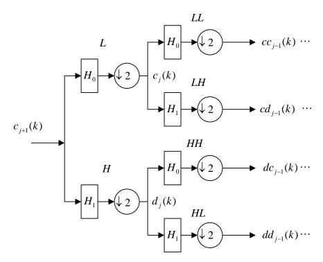
Figure 2.2 Discrete wavelet decomposition for two levels.
