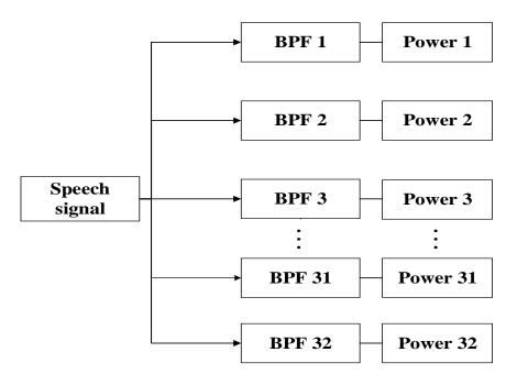
Figure 2.4 Speech decomposition using the bandpass filter banks.
