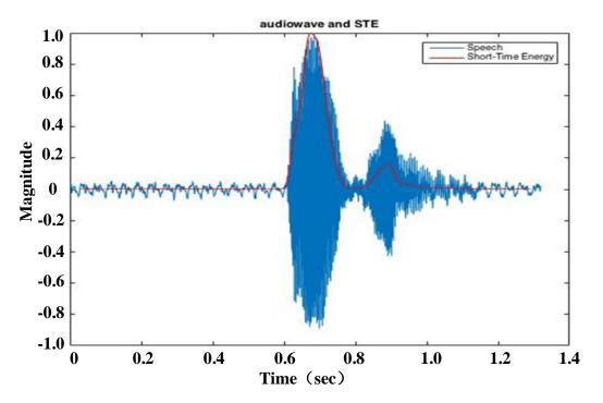
Figure 2.8 Short-term energy and normalized signal ('seven', female).
