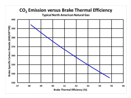
Figure 4.3 BSCO<sub>2</sub> vs Brake Thermal Efficiency
