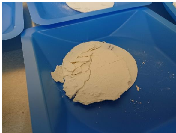
Figure 16 Precipitation collected from YEU supplemented with calcium lactate medium inoculated with L. sphaericus .
