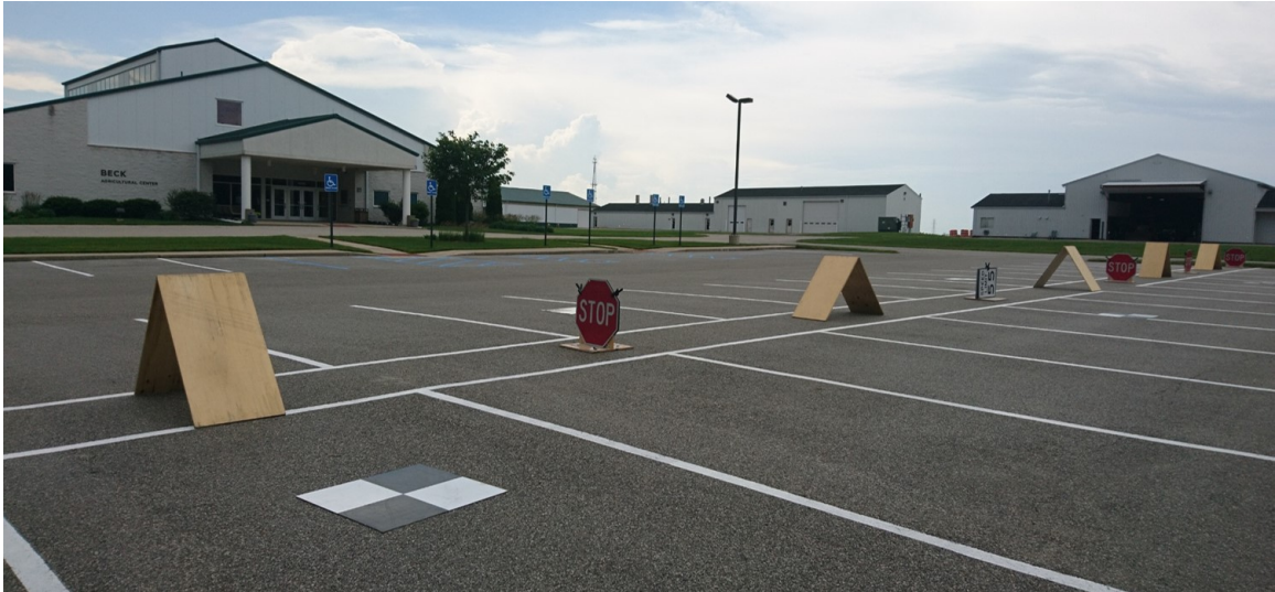
Fig. 4.14.: Calibration test field for the car-mount MMS
