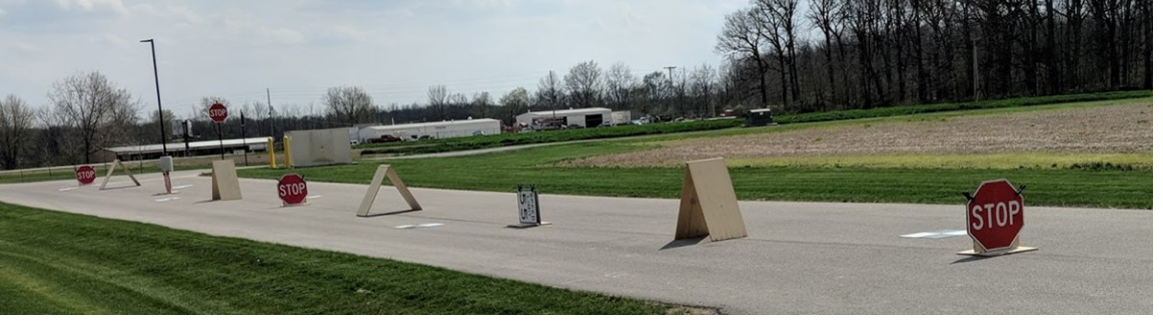
Fig. 4.19.: Calibration test field for the PhenoRover-based MMS
