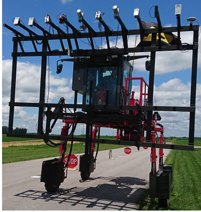
Fig. 4.11.: PhenoRover-based Mobile Mapping System
