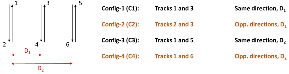
Fig. 3.11.: Drive-run configurations for bias impact analysis
