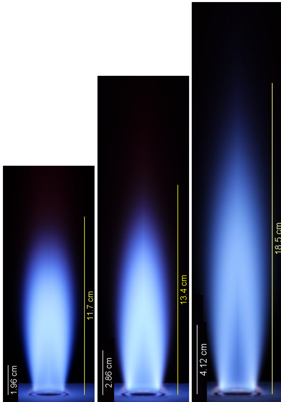
Fig. 4.3. Flame images with 86 % blockage ratio of turbulence generator plate. (left to right: Re 10000, 12500, and 15000)
