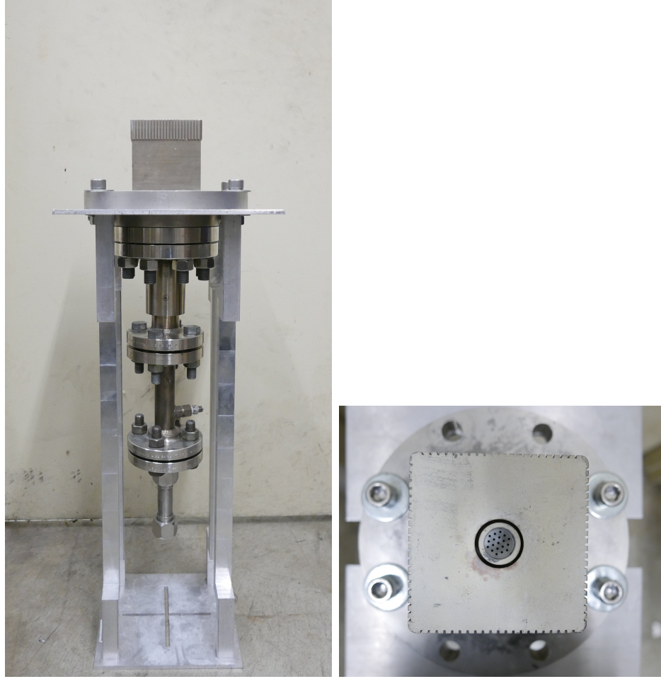
Fig. 3.2. Photographs of PARAT burner. (Left: sideview of PARAT burner. Right: topview of PARAT burner)
