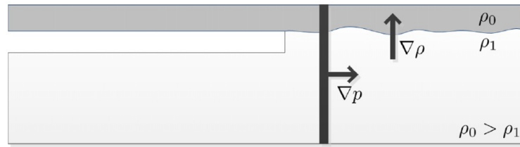
Figure 2.10.: Baroclinic torque action along the shear layer, where the dense fuel is against the wall and the less dense oxidizer in the core. [13]
