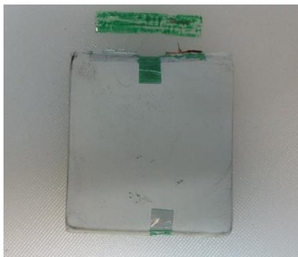
Figure 3.16 Cell Disassembly. Cell after removing the conductive tape along the width of the cell.
