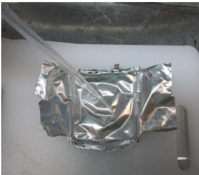
Figure 3.13 Cell Disassembly. IPA poured on the pouch to collect electrolyte.
