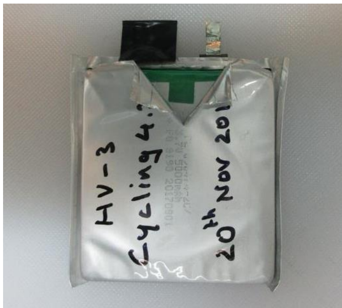
Figure 3.11 Cell Disassembly. Initial cut along the length of the pouch.
