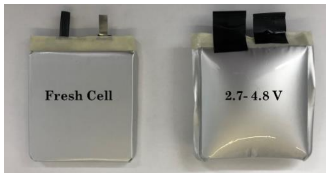
Figure 4.23 Comparison of a fresh cell with a cell cycled in voltage range 2.7 – 4.8 V. The cycled cell under the overcharge condition shows a significant increase in cell swelling.
