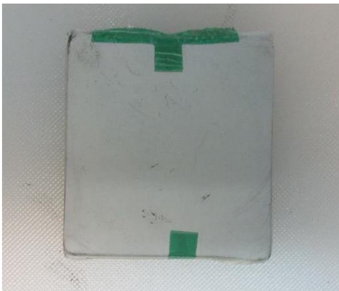
Figure 3.14 Cell Disassembly. Cell before removing the conductive tapes on the separator.
