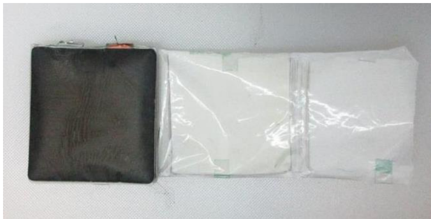
Figure 3.18 Cell Disassembly. Unwinding the separator and extraction of electrodes.
