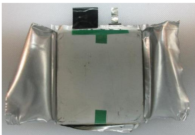
Figure 3.12 Cell Disassembly. Complete cut along the length of the pouch.
