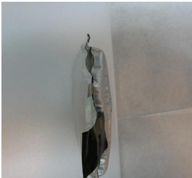
Figure 3.9 Cell disassembly. Initial cut near the tab of the pouch cell.
