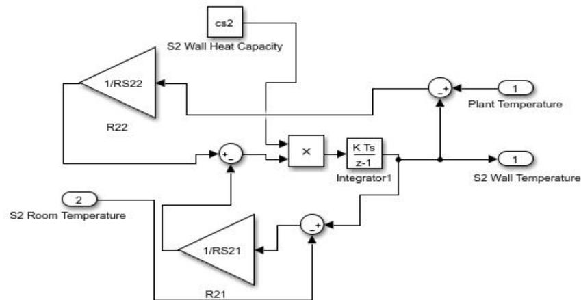
Figure 5.4. Exploded view of the S2 zone wall subsystem. The inputs to this block are the plant temperature and S2 room temperature and the output is the S2 zone wall temperature. R21 and R22 are the thermal resistances, cs2 is the thermal capacity of S2 zone wall
