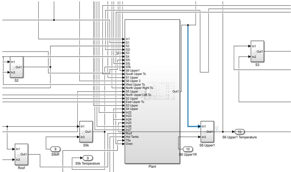
Figure 5.3. Exploded view of the Electro-Spec Plant model showing all the subsystems (zone walls) and disturbances
