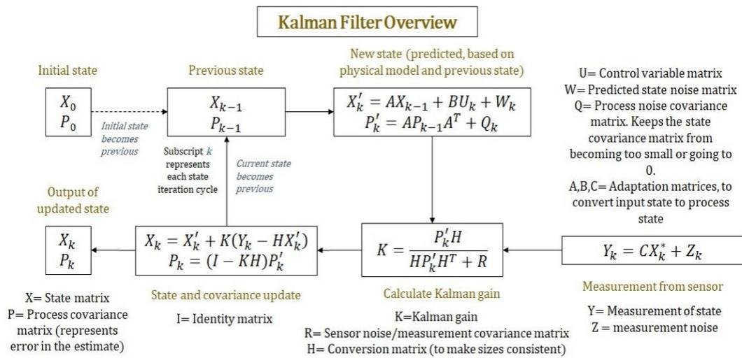
Figure 3.3. Kalman filter process flow chart [31]
