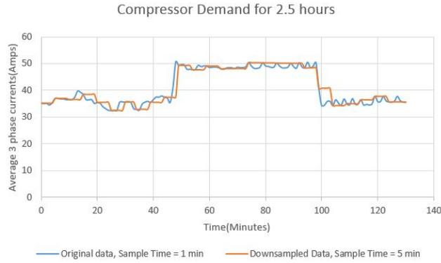
Figure 6.1. Compressor demand data sampled after down sampling
