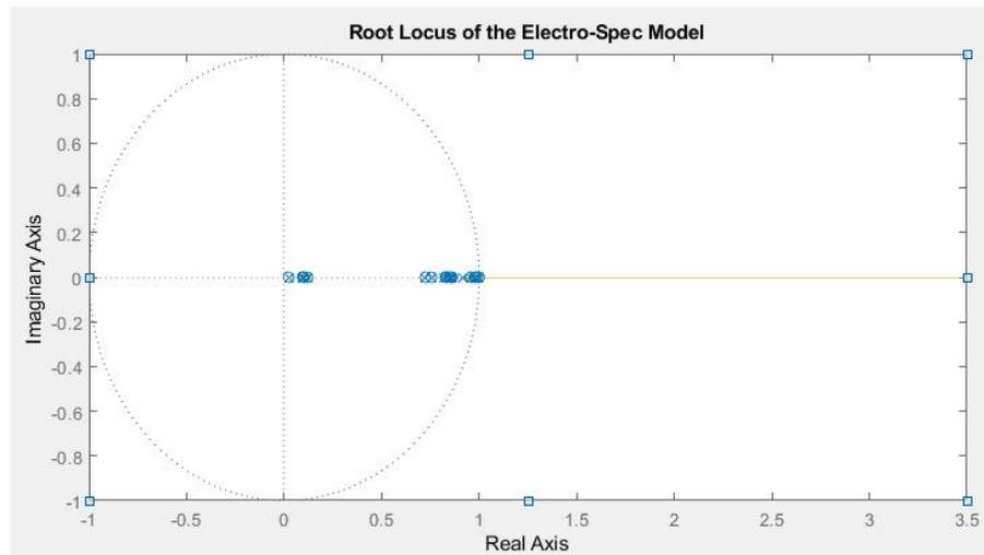
Figure 5.5. Root locus of the Electro-Spec plant model
