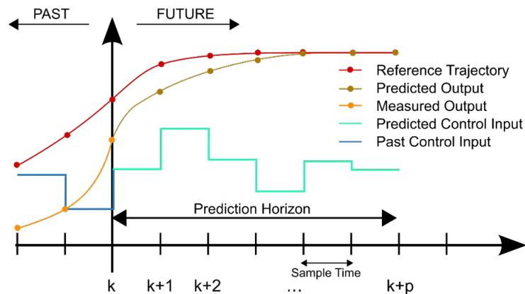
Figure 3.1. Receding horizon control of MPC showing the manipulated and controlled variables
