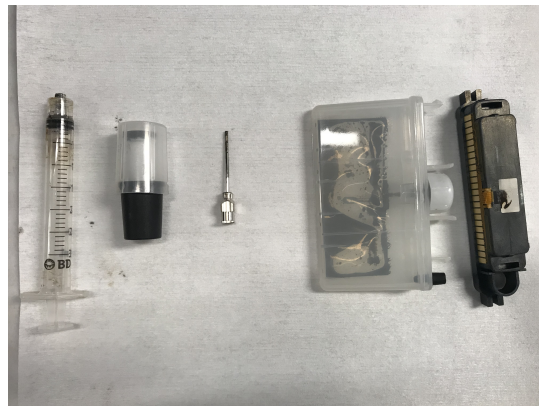
Fig. A.5. Dimatix Disposable Package and Other Accessories (From left to right: syringe, cleansing pad, syringe needle, cartridge with no secure tabs, and jetting model)
