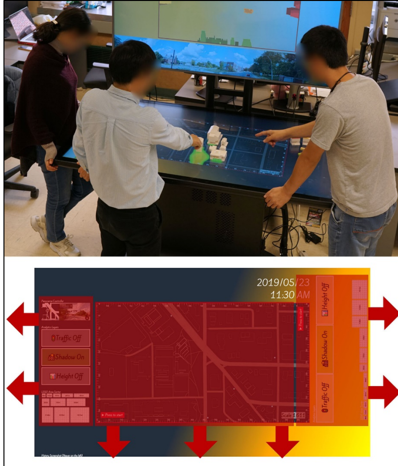
Figure 4.5 Upper: The tabletop interface was designed to be approached in various directions. The maps and panels are serving users from different orientations towards the tabletop, especially for the users from left and right.
