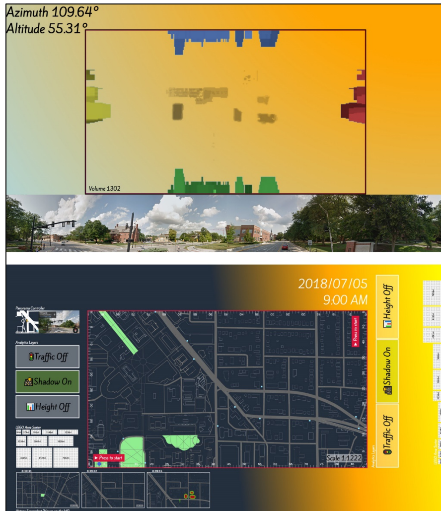
Figure 4.11 Upper: The interface of the information screen. The current information screen (the vertical screen) was showing the depth-cued skylines from four directions. Lower: The interface of the tabletop. The scale and design of the two screens were matched and consistent.
