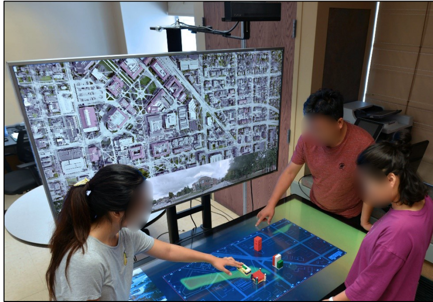
Figure 5.2 The installation set up of the system prototype. The participants were surrounding the tabletop and relocating building blocks to test the changes of impact. The vertical screen was set to a satellite map for peripheral site reference.
