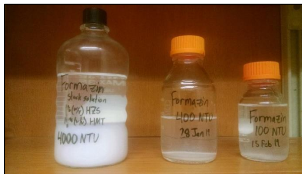
Figure 2: Phase-separated formazin stock suspensions (4000 NTU, 400 NTU, and 100 NTU)
