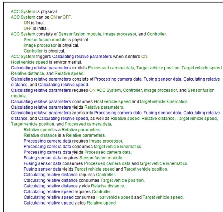
Figure 3.9.: Object-Process Language for SD1.1: ‘Calculating relative parameters’ in-zoomed
