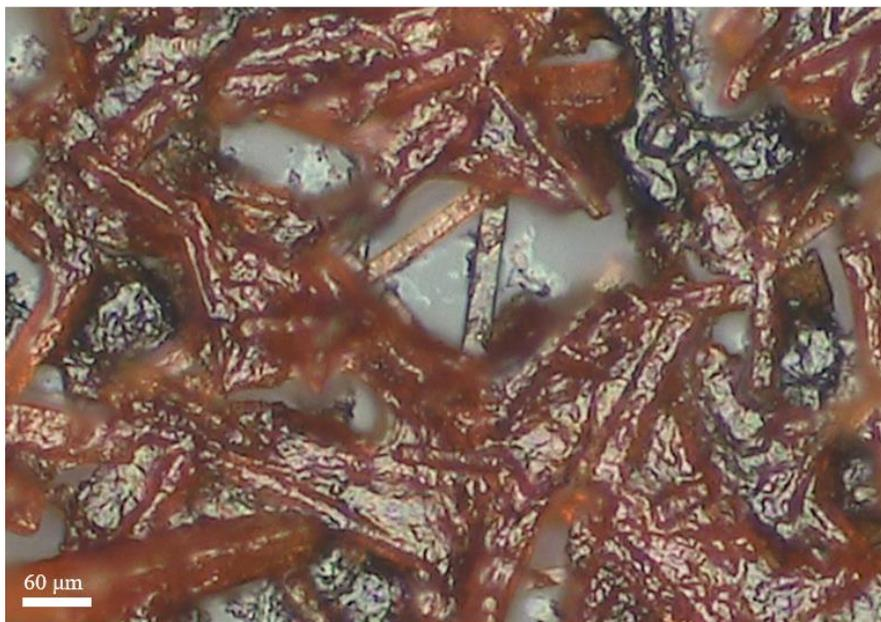
Figure 3.9 Recrystallized BTATz using DMSO as the solvent
