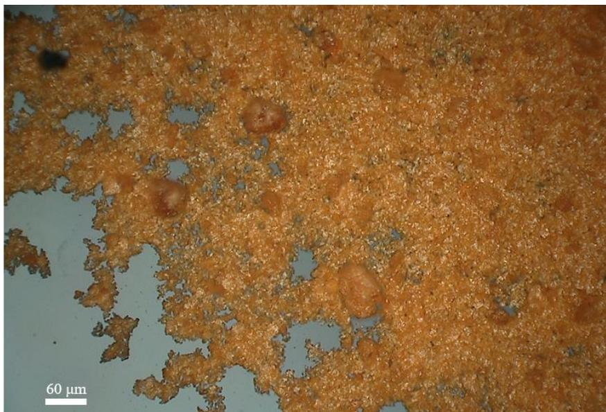
Figure 3.10 Dried BTATz deposited as a suspension with n-hexane
