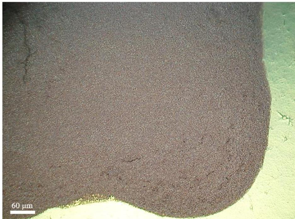
Figure 3.12 Microscopic image of an inkjet printed DAATO<sub>3.5</sub> sample on Novele substrate
