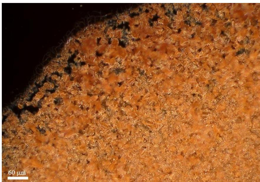
Figure 3.8 Recrystallized BTATz using DMF as the solvent
