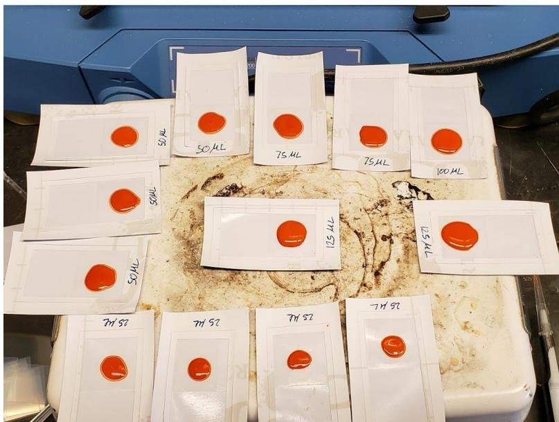
Figure 3.3 Sticker samples drying with varying amounts of deposited BTATz ink
