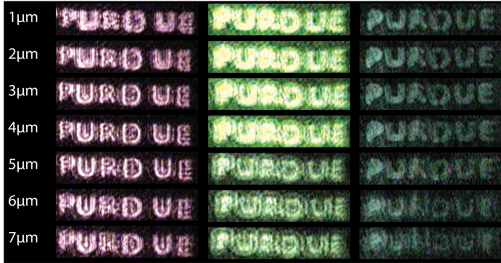
Figure 3.8. Hologram observation by change of focus of the microscope. Left column shows the distance of the focal plane of the microscope set from the surface of the silver film. Each row corresponds to the focal plane for the hologram color
