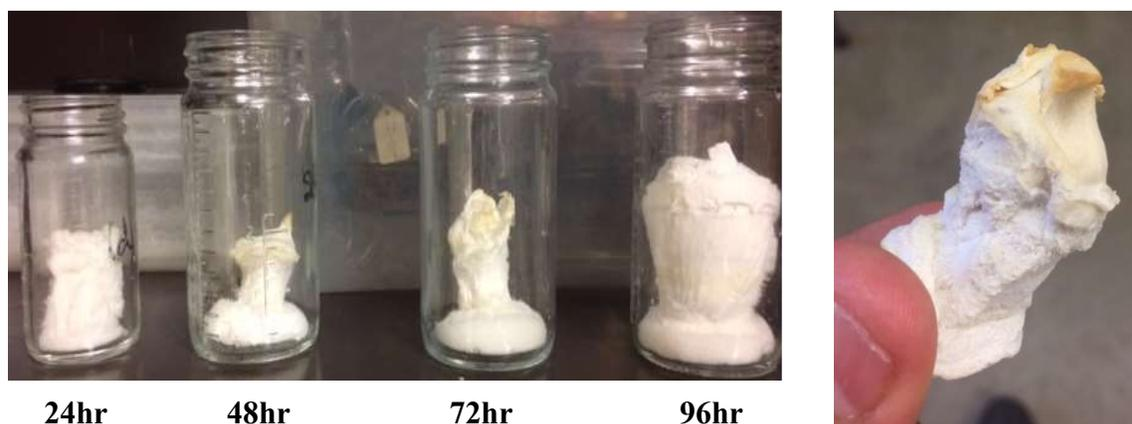
Figure 3.7 *Left*, lyophilized CNF samples taken out at different time periods (1–4 days). *Right*, porous and hardened CNF cake after partial lyophilization then drying under ambient conditions.
