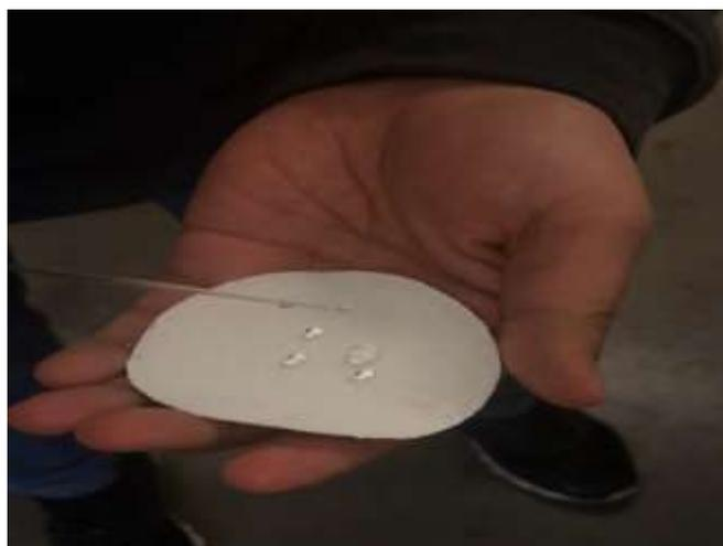
Figure 4.4 Freely moving water droplets on oleylated CNF disk
