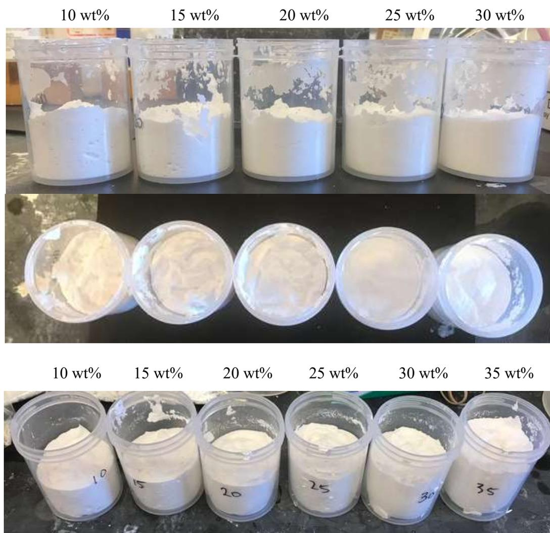
Figure 3.11 CNF cakes after freeze-drying from aqueous slurries containing 10 to 35 wt% TBA.
