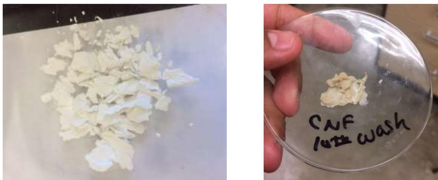
Figure 3.4 Dewatering of acetone-treated CNFs resulted in hardened flakes that resisted further processing
