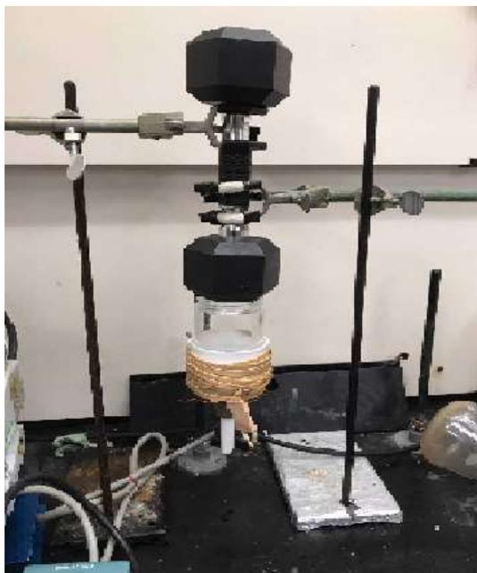
Figure 3.6 Vacuum drying of dewatered CNF samples under a mechanical load
