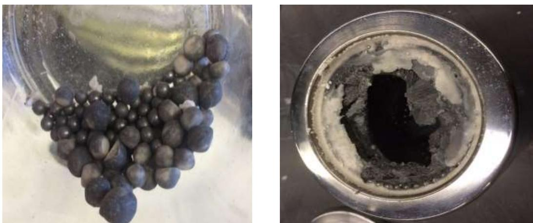
Figure 2.7 MC conditions using a planetary ball mill. Significant degradation or charring of reaction materials was observed.
