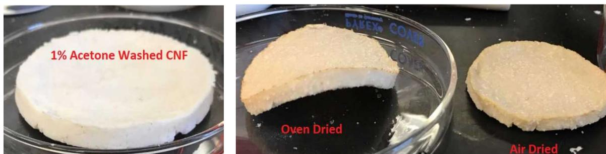
Figure 3.5 Shrinkage and curling of air- and oven-dried CNFs, dewatered by acetone washing
