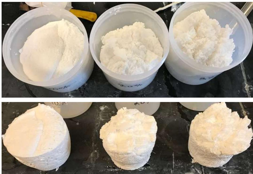
Figure 3.12 Appearance of FD-CNF cakes from aqueous slurries containing 10–30 wt% NBA
