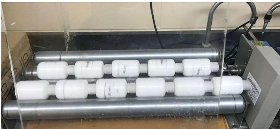
Figure 2.8 Horizontal ball milling with Zr balls in NALGENE bottles (30 rpm)
