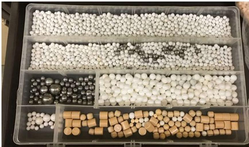
Figure 2.3 Milling media available for mechanochemical grinding
