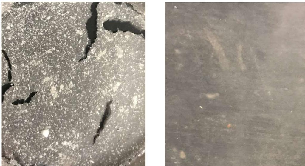
Figure 3.14 Images (5 cm x 5 cm) of cast films prepared from 1 wt% laurylated CNF in chloroform. *Left*, prepared using CNFs lyophilized from water (untreated); *right*, prepared using CNFs lyophilized from slurries with 20 wt% TBA.
