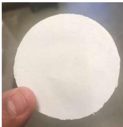
Figure 4.3 *Above*, stearoyl versus oleyl chains grafted on CNF surfaces; *below*, disk of oleyl-CNF after filtering and drying
