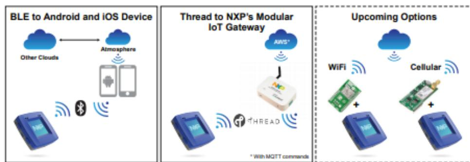
Fig. 3.3. Rapid IoT - System Blocks[30]
