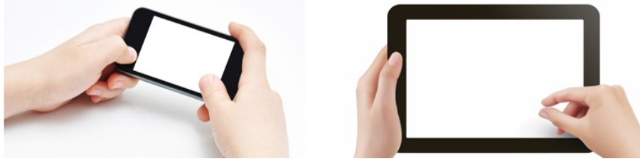
Figure 2.3.: Holding behavior of the control tablet can vary for different sizes of the screen. Small screens are controlled with thumbs, whereas large screens are controlled by one hand.
