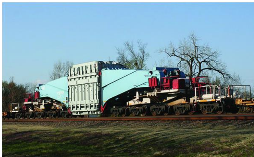
Figure 10. Image of high-voltage transformer being transported in 2008 for Consumers Power using one of only 30 Schnabel rail cars available in the U.S. to transport high-voltage transformers. Retrieved from https://www.powermag.com
